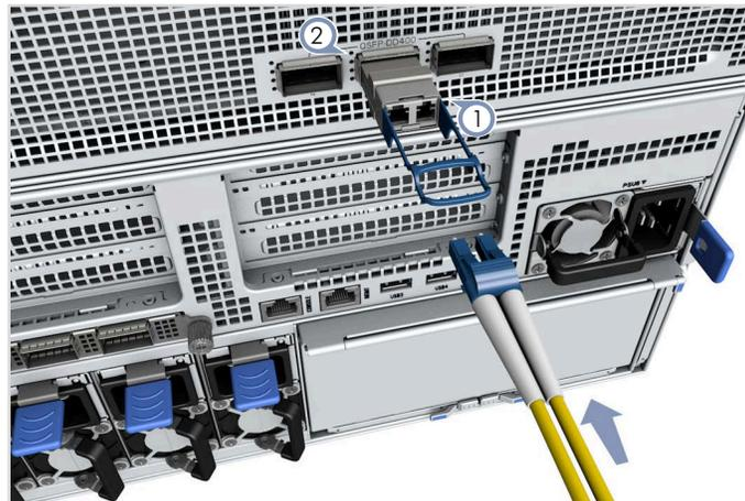
1. QSFP-DD fiber transceiver
