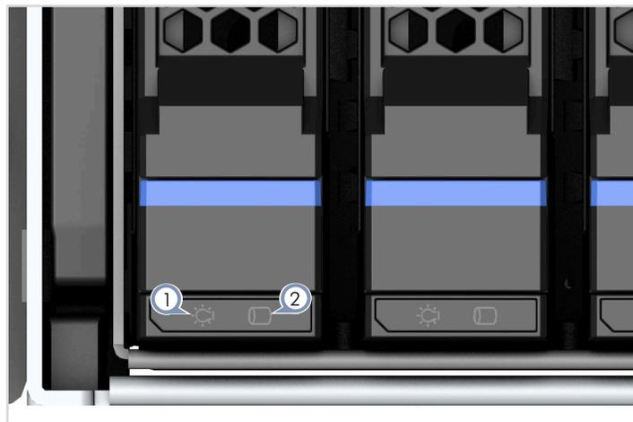
1. HDD/SSD Fault/Locate LED
