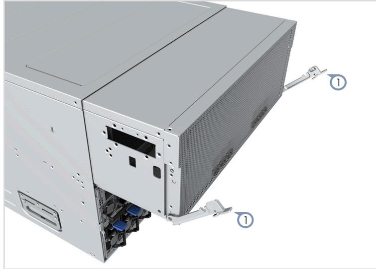
1. GPU module release levers
