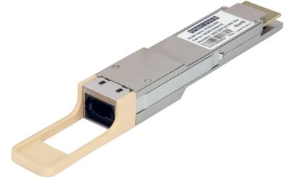
The ET8002-SR8 is an 800G QSFP-DD SR8 transceiver designed to transmit and receive serial optical data up to 106.25 Gbps data rate (per channel) by PAM4 modulation over multimode fiber. It is a small-form-factor hot-pluggable transceiver module integrated with a high-performance VCSEL laser and high-sensitivity PIN receiver. It is compliant with 800G Ethernet and the QSFP-DD MSA.
