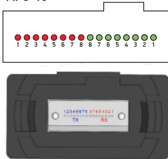
Note: Optical interface is 8°dual APC MPO-16. Lane sequence is shown in the figure above.
