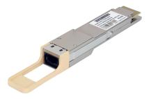
The ET8002-SR8 is an 800G QSFP-DD SR8 transceiver designed to transmit and receive serial optical data up to 106.25 Gbps data rate (per channel) by PAM4 modulation over multimode fiber. It is a small-form-factor hot-pluggable transceiver module integrated with a high-performance VCSEL laser and high-sensitivity PIN receiver. It is compliant with 800G Ethernet and the QSFP-DD MSA.
