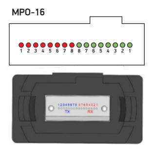
Note: Optical interface is 8°dual APC MPO-16. Lane sequence is shown in the figure above.
