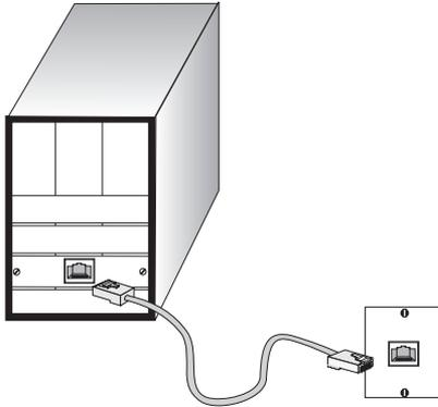
2. If the device is a network card and the switch is in the wiring closet, attach the other end of the cable segment to a modular wall outlet that is connected to the wiring closet. Otherwise, attach the other end to an available port on the switch.
