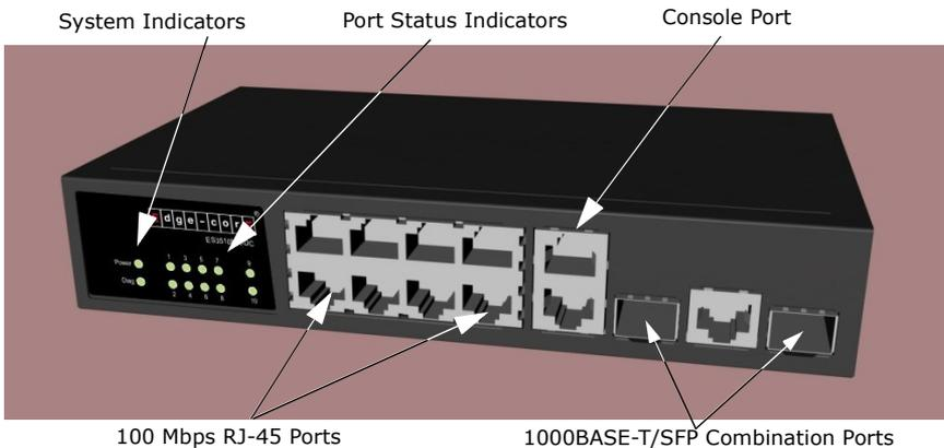
1. If an SFP transceiver is plugged in, the corresponding RJ-45 port is disabled for ports 9-10.
