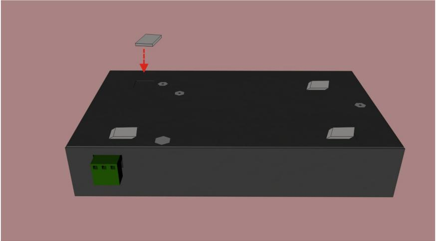
2. Set the device on a flat surface near an AC power source, making sure there are at least two inches of space on all sides for proper air flow.
