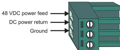
6. Insert the wire leads into the openings shown in the figure above. Each lead inserted in the power plug must match the lead attached to the power source. Use the labeling above the DC power connector to identify the appropriate power input and return or ground lines.
