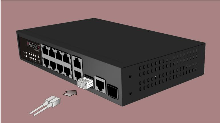
4. As a connection is made, check the Link LED on the switch corresponding to the port to be sure that the connection is valid.
