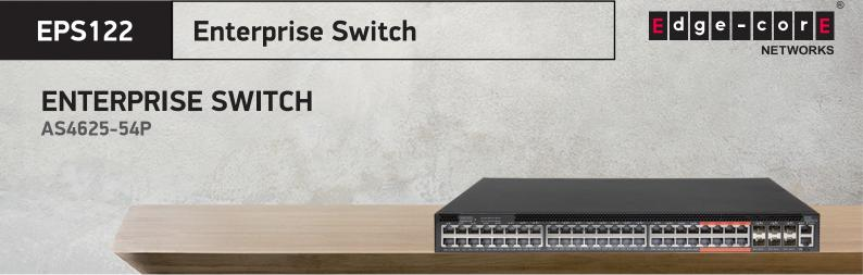
The Edgecore EPS122 is a cost-effective, high-performance Gigabit Ethernet L2 PoE switch featuring 54 ports; 48 x 10/100/1000BASE-T ports and 6 x 1G/10G SFP+ uplink ports. Ports 1 to 40 (10/100/1000BASE-T) fully support IEEE 802.3at and IEEE 802.3bt Power-over-Ethernet (PoE) up to 30 W, and ports 41 to 48 (10/100/1000BASE-T) fully support IEEE 802.3at and IEEE 802.3bt Type 4 up to 90 W.
