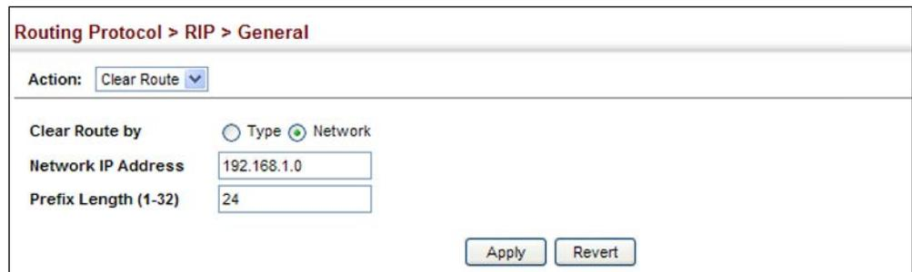
The screenshot shows a web interface for configuring the Routing Information Protocol (RIP). The breadcrumb path is "Routing Protocol > RIP > General". The "Action" dropdown menu is set to "Clear Route". Under the "Clear Route by" section, the "Network" radio button is selected. The "Network IP Address" field contains "192.168.1.0" and the "Prefix Length (1-32)" field contains "24". At the bottom right, there are "Apply" and "Revert" buttons.
