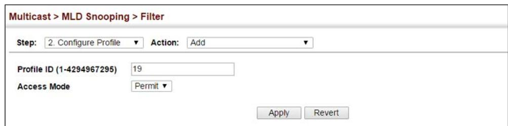
The screenshot shows a web interface for configuring an MLD filter profile. The breadcrumb path is "Multicast > MLD Snooping > Filter". The "Step" dropdown is set to "2. Configure Profile" and the "Action" dropdown is set to "Add". The "Profile ID (1-4294967295)" field contains the value "19". The "Access Mode" dropdown is set to "Permit". At the bottom right, there are "Apply" and "Revert" buttons.
