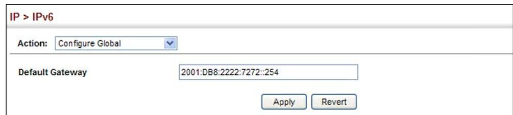
The screenshot shows a web interface for configuring IPv6 settings. At the top, it says "IP > IPv6". Below that, there is a dropdown menu for "Action" set to "Configure Global". Underneath, there is a text input field for "Default Gateway" containing the address "2001:DB8:2222:7272::254". At the bottom right of the form, there are two buttons: "Apply" and "Revert".
