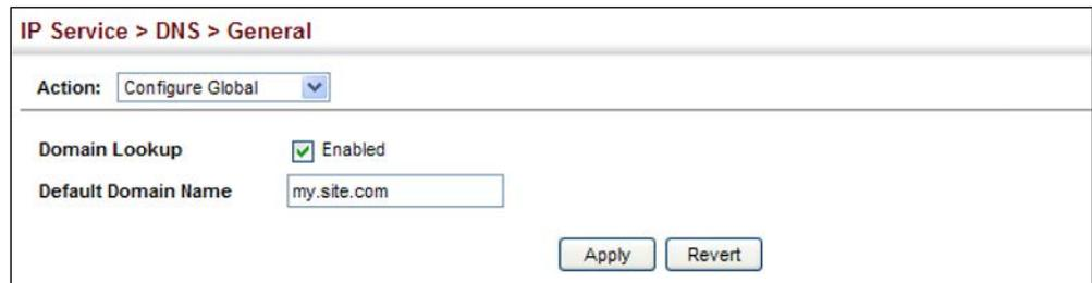
The screenshot shows a web interface for configuring DNS settings. The breadcrumb path is "IP Service > DNS > General". Below the breadcrumb, there is an "Action:" dropdown menu currently set to "Configure Global". Underneath, there are two configuration items: "Domain Lookup" with a checked checkbox and the text "Enabled", and "Default Domain Name" with a text input field containing "my.site.com". At the bottom right of the configuration area, there are two buttons: "Apply" and "Revert".
