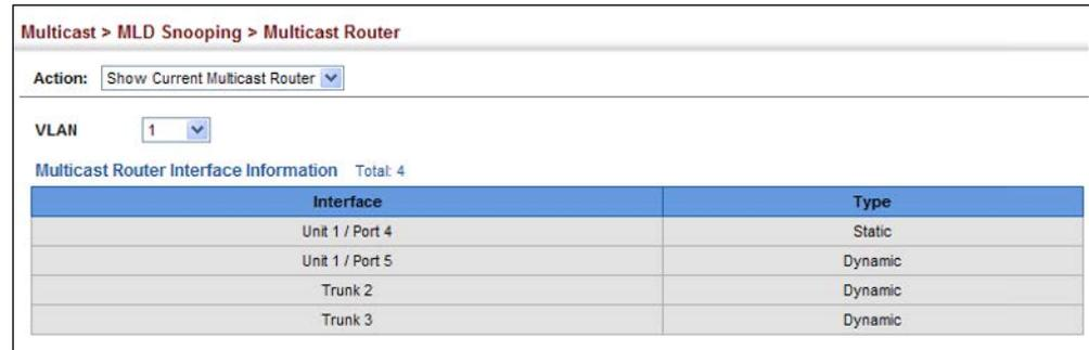
Multicast > MLD Snooping > Multicast Router
