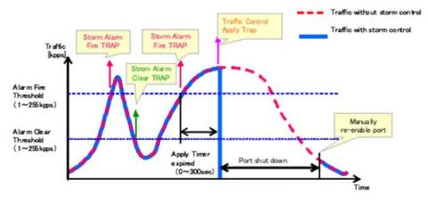
Figure 2: Storm Control by Shutting Down a Port
