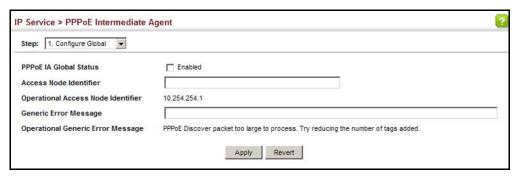
Configuring PPPoE IA Use the IP Service > PPPoE Intermediate Agent (Configure Interface) page to enable Interface Settings PPPoE IA on an interface, set trust status, enable vendor tag stripping, and set the circuit ID and remote ID.
