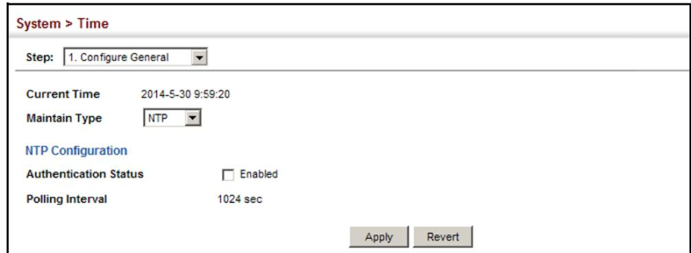
The screenshot shows a web interface for configuring NTP. At the top, it says "System > Time". Below that, there is a "Step:" dropdown menu set to "1. Configure General". The "Current Time" is displayed as "2014-5-30 9:59:20". The "Maintain Type" is set to "NTP" via a dropdown menu. Under the "NTP Configuration" section, the "Authentication Status" is "Enabled" with an unchecked checkbox. The "Polling Interval" is set to "1024 sec". At the bottom right, there are "Apply" and "Revert" buttons.
