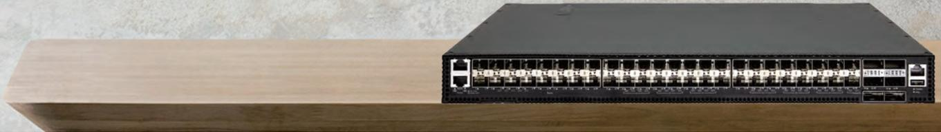
The Edgecore DCS201 switch meets the high-performance, availability, and network-scaling requirements of enterprise and cloud data centers. The DCS201 provides full line-rate switching at Layer 2 or Layer 3 across 48 x 10GbE ports and 6 x 100GbE uplinks. The switch can be deployed either as a top-of-rack switch, or as part of a 40GbE or 100GbE distributed spine, forming a non-blocking folded-Clos data center fabric. The switch is rack mountable in a standard 19-inch rack.
