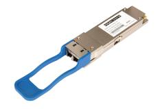
The ET7402-LR1 100G QSFP28 LR transceiver is designed to provide a convenient solution for 100G applications in a QSFP28 form factor. The QSFP28 LR transceiver supports a single 53.125 GBd optical lane and is designed for uses up to a 106.25 Gb/s data rate and up to a 10 km link length. The transceiver supports an I2C and digital diagnostic management (DDM) interface.
