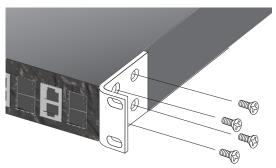
**2.** Mount the device in the rack, using four rack-mounting screws (not provided).
