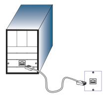
2. If the device is a PC card and the switch is in the wiring closet, attach the other end of the cable segment to a modular wall outlet that is connected to the wiring closet. (See "Network Wiring Connections" on page 47.)
