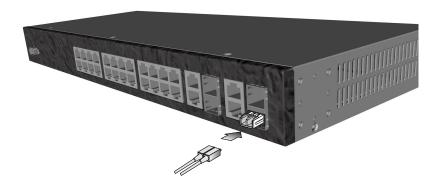
**4.** As a connection is made, check the Link LED on the switch corresponding to the port to be sure that the connection is valid.
