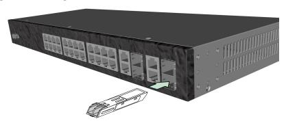
The switch supports 1000BASE-SX, 1000BASE-LX, 1000BASE-LH and other SFP-compatible transceivers. To install an SFP transceiver, do the following:
