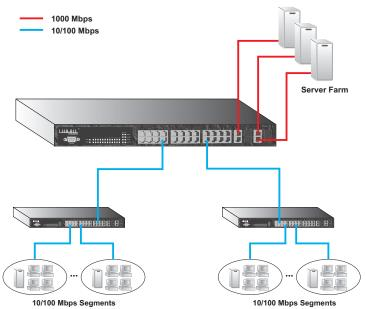
Figure 6: Network Aggregation Plan
