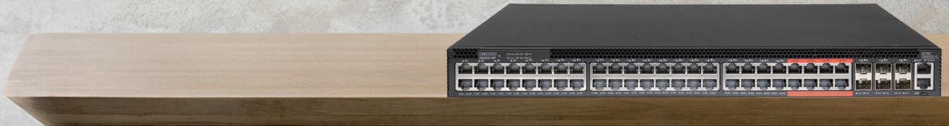
The Edgecore EPS122 is a cost-effective, high-performance Gigabit Ethernet L2 PoE switch featuring 54 ports; 48 x 10/100/1000BASE-T ports and 6 x 1G/10G SFP+ uplink ports. Ports 1 to 40 (10/100/1000BASE-T) fully support IEEE 802.3at and IEEE 802.3bt Power-over-Ethernet (PoE) up to 30 W, and ports 41 to 48 (10/100/1000BASE-T) fully support IEEE 802.3at and IEEE 802.3bt Type 4 up to 90 W.
