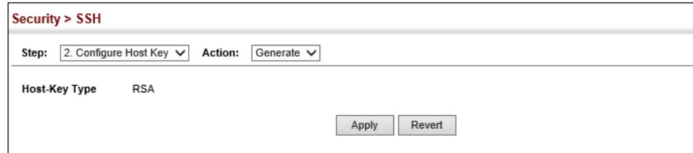
Figure 204: Generating the SSH Host Key Pair
