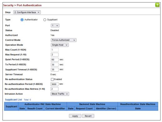
Figure 223: Configuring Interface Settings for 802.1X Port Authenticator
