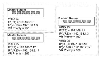
Figure 514: Several Virtual Master Routers Configured for Mutual Backup and Load Sharing
