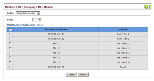
To display information about all IPv6 multicast groups, MLD Snooping or multicast routing must first be enabled on the switch. To show all of the interfaces statically or dynamically assigned to an IPv6 multicast service:
