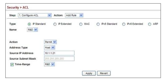
Configuring an Use the Security > ACL (Configure ACL - Add Rule - IP Extended) page to configure Extended IPv4 ACL an Extended IPv4 ACL.
