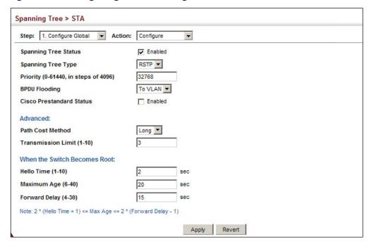
Figure 126: Configuring Global Settings for STA (MSTP)
