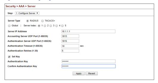
**Figure 175: Configuring Remote Authentication Server** (TACACS+)
