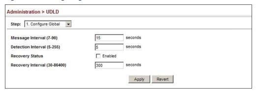
Configuring UDLD Use the Administration > UDLD (Configure Interface) page to enable UDLD and Interface Settings aggressive mode which reduces the shut-down delay after loss of bidirectional connectivity is detected.
