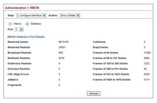
**Figure 308: Showing Collected RMON Statistical Samples**
