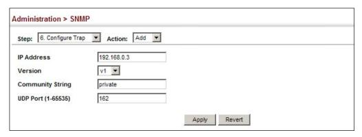
**Figure 293: Configuring Trap Managers** (SNMPv2c)
