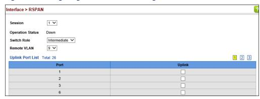
Figure 66: Configuring Remote Port Mirroring (Destination)
