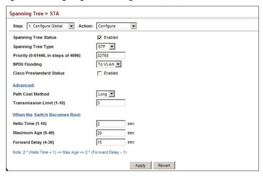
Figure 125: Configuring Global Settings for STA (RSTP)
