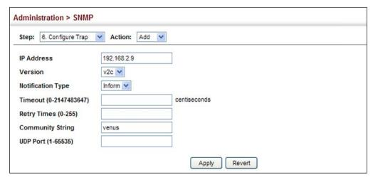
Figure 294: Configuring Trap Managers (SNMPv3)
