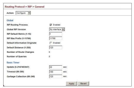
Clearing Entries from Use the Routing Protocol > RIP > General (Clear Route) page to clear entries from the Routing Table the routing table based on route type or a specific network address.
