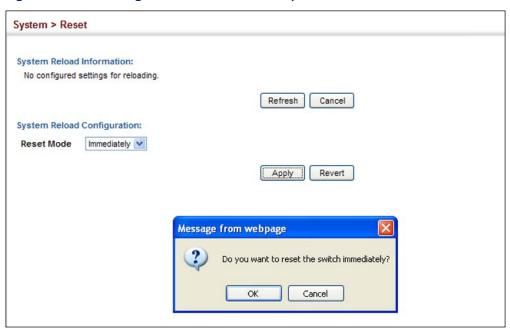
Figure 27: Restarting the Switch (In)
