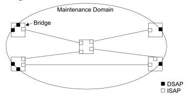
**Figure 334: Single CFM Maintenance Domain**
