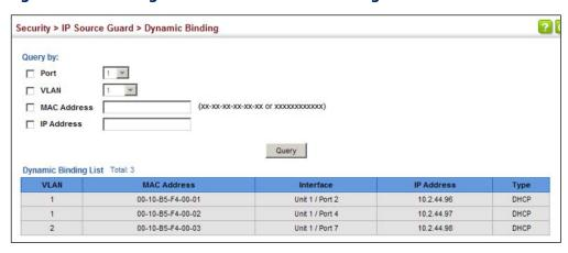
Figure 246: Showing the IPv4 Source Guard Binding Table
