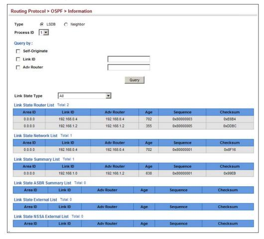
Figure 563: Displaying Information in the Link State Database
