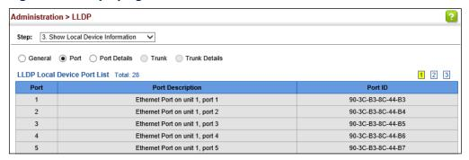
Figure 267: Displaying Local Device Information for LLDP (Port Details)
