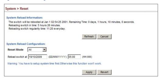
Figure 29: Restarting the Switch (Regularly)
