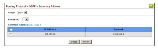
**Configuring OSPF** You should specify a routing interface for any local subnet that needs to Interfaces communicate with other network segments located on this router or elsewhere in the network. First configure a VLAN for each subnet that will be directly connected to this router, assign IP interfaces to each VLAN (i.e., one primary interface and one or more secondary interfaces), and then use the Network Area configuration page to assign an interface address range to an OSPF area.
