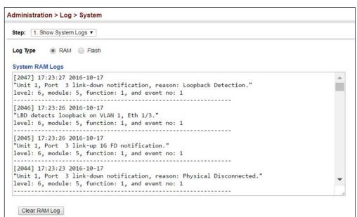
Figure 258: Showing Error Messages Logged to System Memory
