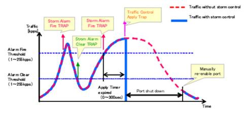
Figure 4: Storm Control by Shutting Down a Port
