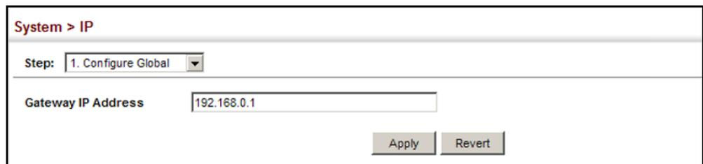
The screenshot shows a web interface for configuring the switch's IP. The breadcrumb navigation is "System > IP". Below this, there is a "Step:" dropdown menu currently set to "1. Configure Global". The main configuration area has a label "Gateway IP Address" followed by a text input field containing the value "192.168.0.1". At the bottom right of the form are two buttons: "Apply" and "Revert".
