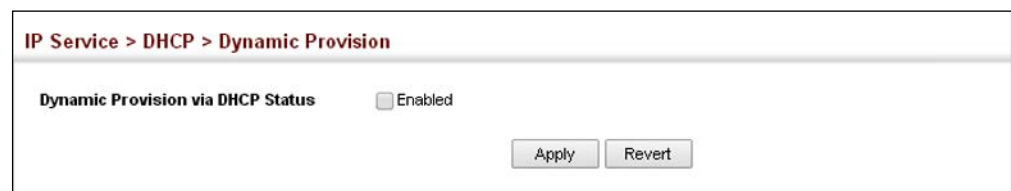
Figure 485: Enabling Dynamic Provisioning via DHCP
