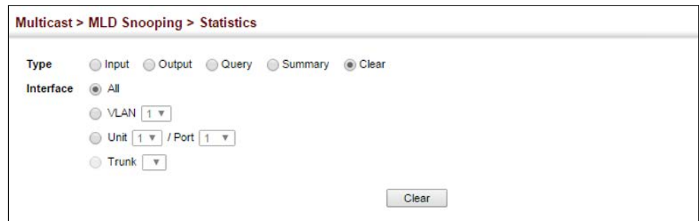
Figure 410: Clearing MLD Snooping Statistics
