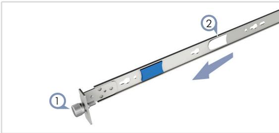
1. For each rack-rail assembly, pull the slide-rail out to its full extended position.
