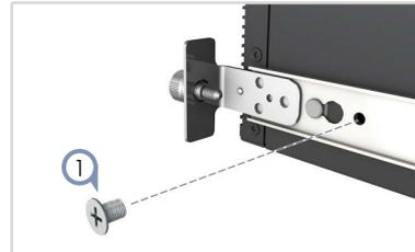
1. Unscrew and remove the M4 security screws from the inner rails.
