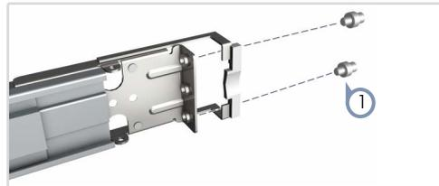
1. Replace the rack hole pins on the rail assemblies for “round-hole” rack posts. Tighten the pins to a torque of 20-25 Kgf-cm. (Rack square hole pins are pre-installed.)
