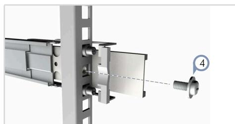
4. Secure each rail assembly to the rear post using the included M5 rack screws. Tighten the screws to a torque of 20-25 Kgf-cm.
