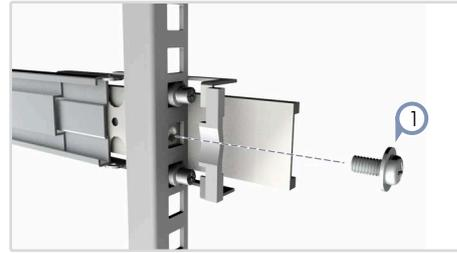
1. Unscrew and remove the rear post M5 rack screws from each rail assembly.
