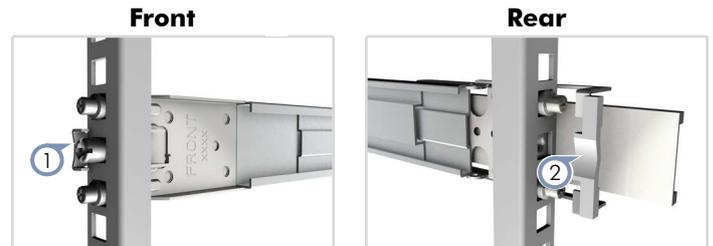
2. At the front of each rack-rail assembly, pull the lever to release the assembly from the front rack post.
