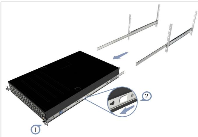
1. Unscrew both thumb screws on the inner rails and slide the chassis out to its full extended locked position.
