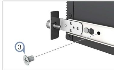
3. Use the M4 screws to provide additional security for the inner rail attachment to the switch. Tighten the screws to a torque of 15-20 Kgf-cm.
