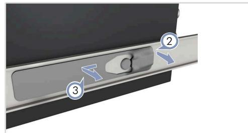
2. At the rear end of each inner rail, pull up the spring latch to release the rail from the switch stand-offs.
