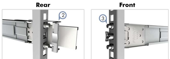
2. For each rack-rail assembly, attach the rear part of the rails to the rear rack posts.
