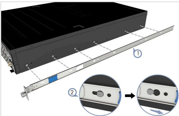
1. Position each inner slide-rail on the side of the switch so that it aligns with the six mounting stand-offs.
