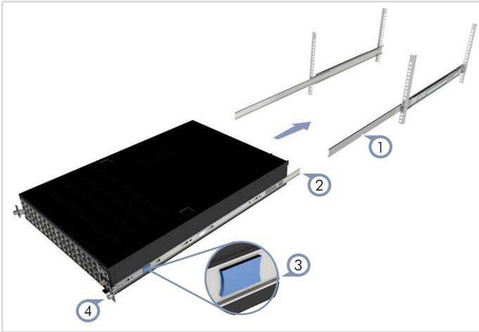
1. Pull the middle rails out to their full extended locked position. Ensure the inner ball bearing retainers are located at the front of the middle rails.
