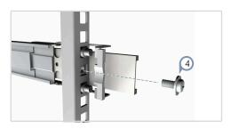
**4.** Secure each rail assembly to the rear post using the included M5 rack screws. Tighten the screws to a torque of 20-25 Kgf-cm.
