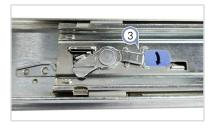
3. Push the lever on the middle rails to retract them back into the rail assemblies.
