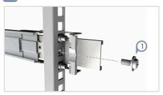
1. Unscrew and remove the rear post M5 rack screws from each rail assembly.
