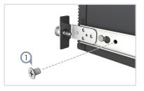
1. Unscrew and remove the M4 security screws from the inner rails.
