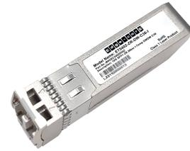
Edgecore's ET5402-ZR-DW transceiver module is designed for C-band DWDM 10G Ethernet links over 80km single mode fiber. The module incorporates a DWDM Electro-absorption Modulated Laser (EML) transmitter in the C-band channel (Cxy) and an avalanche photodiode (APD) receiver. The electrical interface of the module is compliant with the SFP+ MSA. Digital diagnostic functions are available via a 2-wire serial interface, as specified in SFF-8472.
