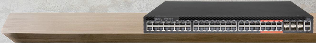
The Edgecore EPS122 is a cost-effective, high-performance Gigabit Ethernet L2 PoE switch featuring 54 ports; 48 x 10/100/1000BASE-T ports and 6 x 1G/10G SFP+ uplink ports. Ports 1 to 40 (10/100/1000BASE-T) fully support IEEE 802.3at and IEEE 802.3bt Power-over-Ethernet (PoE) up to 30 W, and ports 41 to 48 (10/100/1000BASE-T) fully support IEEE 802.3at and IEEE 802.3bt Type 4 up to 90 W.
