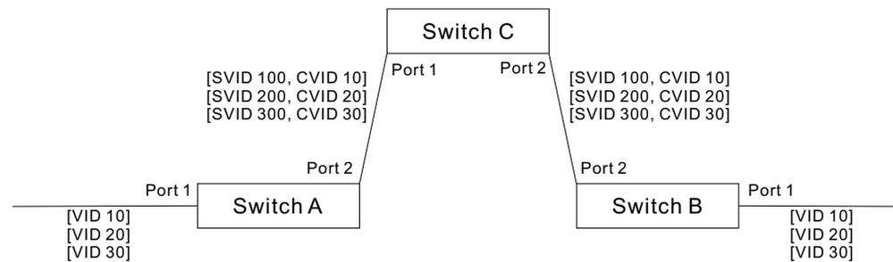
Step 1. Configure Switch A and B.
