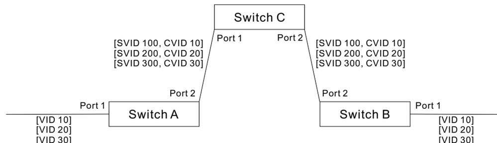
Step 1. Configure Switch A and B.
