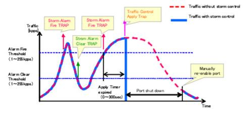
Figure 2: Storm Control by Shutting Down a Port
