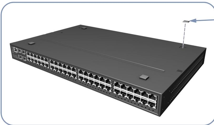
Attach the four adhesive rubber foot pads to the recessed areas on the bottom of the switch.
