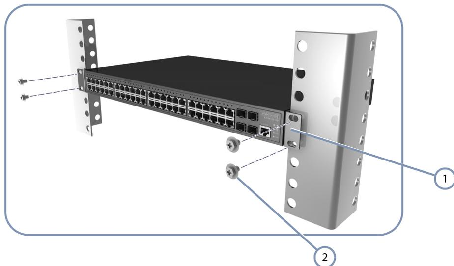
1 Attach the brackets to the switch,
