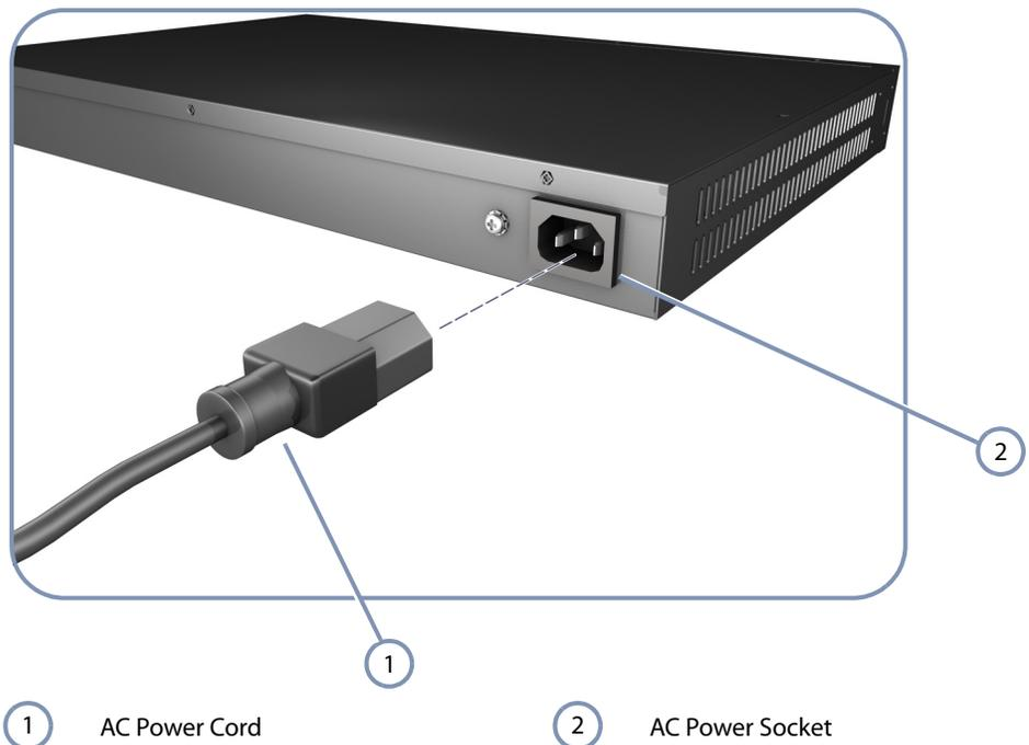
2. Insert the plug on the other end of the power cord directly into the AC input socket on the back of the switch.
