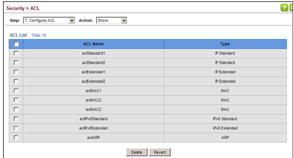
**Configuring a Standard IPv4 ACL** Use the Security > ACL (Configure ACL - Add Rule - IP Standard) page to configure a Standard IPv4 ACL.
