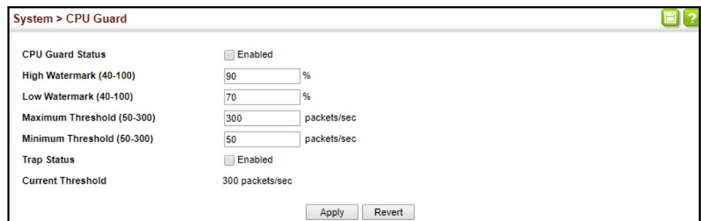
The screenshot shows a web interface for configuring CPU Guard. The breadcrumb path is "System > CPU Guard". The configuration options are as follows:
