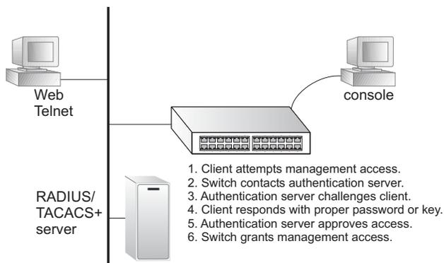
RADIUS uses UDP while TACACS+ uses TCP. UDP only offers best effort delivery, while TCP offers a more reliable connection-oriented transport. Also, note that
