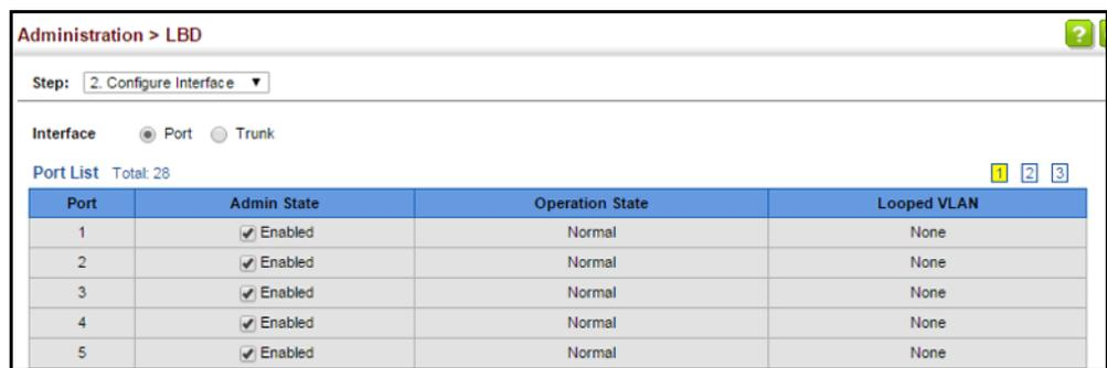
The screenshot shows the 'Administration > LBD' configuration page. The 'Step' is '2. Configure Interface'. Under 'Interface', the 'Port' radio button is selected. Below is a 'Port List' table with 5 rows and 4 columns: Port, Admin State, Operation State, and Looped VLAN. All ports are listed as 'Enabled' and 'Normal' with 'None' for the Looped VLAN.
