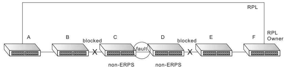
When non-ERPS device protection is enabled on the ring, the ring ports on the RPL owner node and non-owner nodes will not be blocked when signal loss is detected by CCM loss events.
