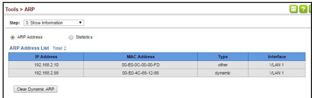
**Displaying ARP Statistics** Use the Tools > ARP (Show Information) page to display statistics for ARP messages crossing all interfaces on this switch.
