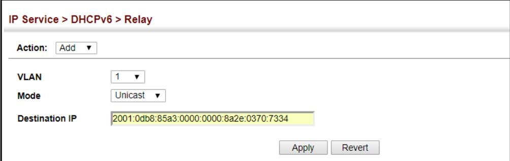
The screenshot shows a web interface for configuring DHCPv6 Relay. The breadcrumb navigation is "IP Service > DHCPv6 > Relay". Below the breadcrumb, there is an "Action:" dropdown menu set to "Add". The "VLAN" field is a dropdown menu set to "1". The "Mode" field is a dropdown menu set to "Unicast". The "Destination IP" field is a text input containing the IPv6 address "2001:0db8:85a3:0000:0000:8a2e:0370:7334". At the bottom right, there are two buttons: "Apply" and "Revert".
