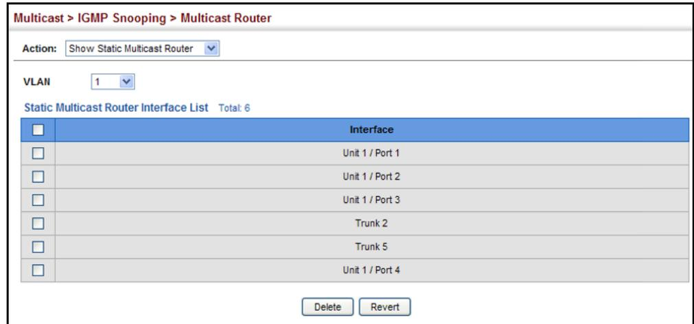
Multicast routers that are attached to ports on the switch use information obtained from IGMP, along with a multicast routing protocol (such as PIM) to support IP multicasting across the Internet. These routers may be dynamically discovered by the switch or statically assigned to an interface on the switch.
