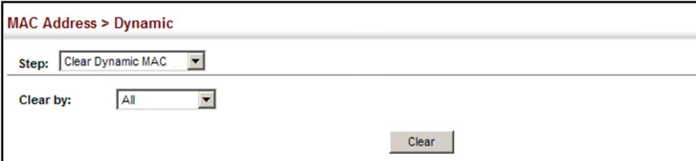
The screenshot shows a web interface for clearing dynamic MAC address table entries. The breadcrumb path is "MAC Address > Dynamic". There are two dropdown menus: "Step:" with "Clear Dynamic MAC" selected, and "Clear by:" with "All" selected. A "Clear" button is located at the bottom right of the form.
