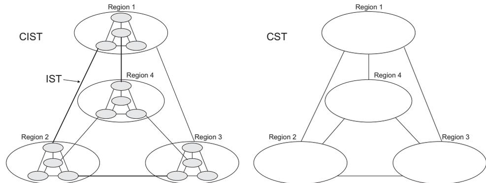
MSTP connects all bridges and LAN segments with a single Common and Internal Spanning Tree (CIST). The CIST is formed as a result of the running spanning tree algorithm between switches that support the STP, RSTP, MSTP protocols.
