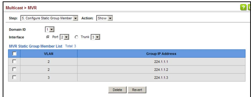
**Displaying MVR Receiver Groups** Use the Multicast > MVR (Show Member) page to show the multicast groups either statically or dynamically assigned to the MVR receiver groups on each interface.
