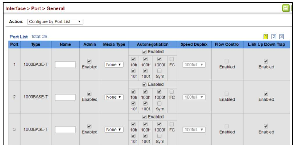
**Configuring by Port Range** Use the Interface > Port > General (Configure by Port Range) page to enable/disable an interface, set auto-negotiation and the interface capabilities to advertise, or manually fix the speed, duplex mode, and flow control.
