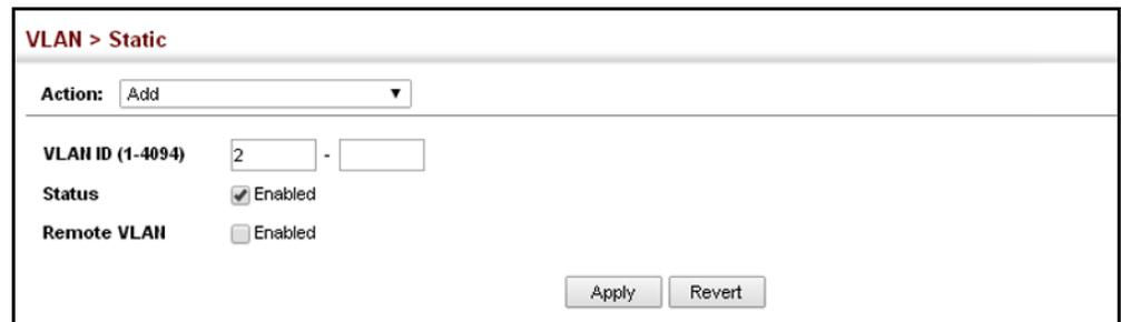
The screenshot shows a web interface for configuring static VLANs. At the top, it says "VLAN > Static". Below that is an "Action:" dropdown menu with "Add" selected. The main configuration area has three rows: "VLAN ID (1-4094)" with input boxes containing "2" and a hyphen; "Status" with a checked checkbox and the text "Enabled"; and "Remote VLAN" with an unchecked checkbox and the text "Enabled". At the bottom right, there are two buttons: "Apply" and "Revert".
