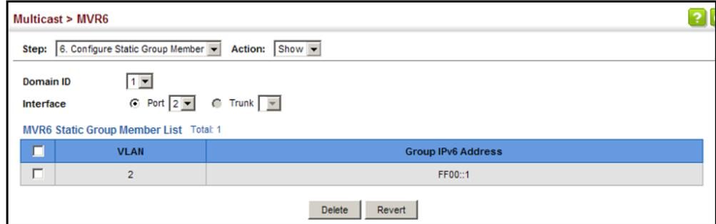
**Displaying MVR6 Receiver Groups** Use the Multicast > MVR6 (Show Member) page to show the multicast groups either statically or dynamically assigned to the MVR6 receiver groups on each interface.
