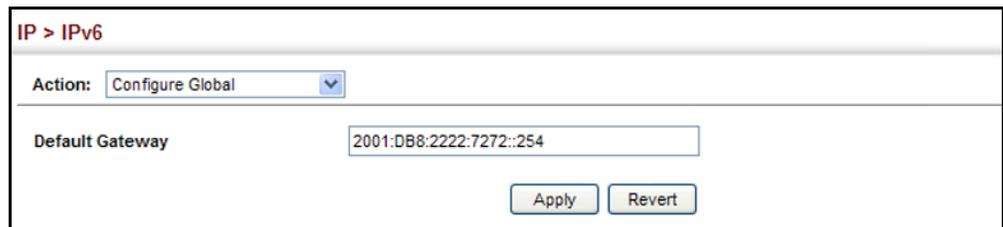
The screenshot shows a web interface for configuring IPv6 settings. At the top, the breadcrumb is "IP > IPv6". Below that, there is a dropdown menu for "Action" currently set to "Configure Global". Underneath, there is a text input field for "Default Gateway" containing the address "2001:0B8:2222:7272::254". At the bottom right of the form, there are two buttons: "Apply" and "Revert".
