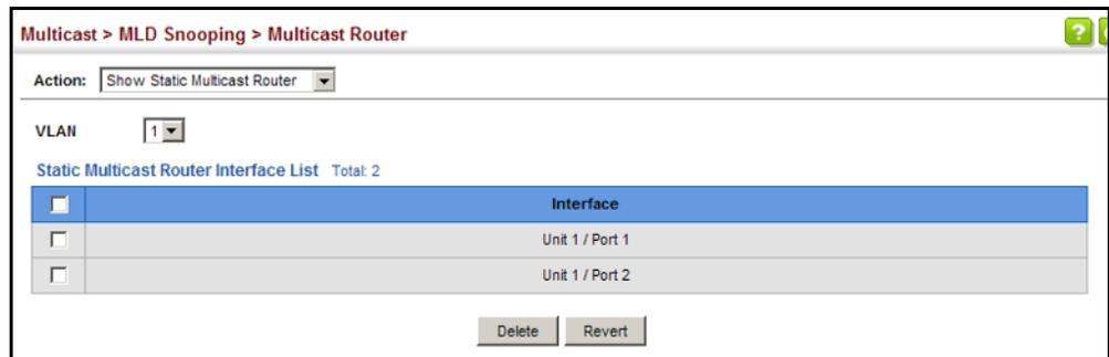
To show all the interfaces attached to a multicast router:
