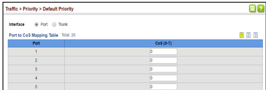
The screenshot shows a web interface for configuring queue settings. The breadcrumb path is 'Traffic > Priority > Default Priority'. There are two radio buttons for 'Interface': 'Port' (selected) and 'Trunk'. Below this is a 'Port to CoS Mapping Table' with a 'Total: 26' and three numbered tabs (1, 2, 3). The table has two columns: 'Port' and 'CoS (0-7)'. The 'CoS' column contains input fields with the value '0'.
