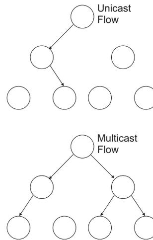
This switch can use Internet Group Management Protocol (IGMP) to filter multicast traffic. IGMP Snooping can be used to passively monitor or “snoop” on exchanges between attached hosts and an IGMP-enabled device, most commonly a multicast router. In this way, the switch can discover the ports that want to join a multicast group, and set its filters accordingly.
