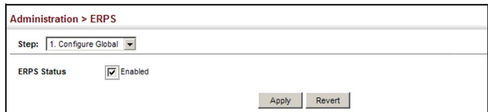
The screenshot shows a web interface for configuring ERPS. At the top, it says "Administration > ERPS". Below that, there is a "Step:" dropdown menu with "1. Configure Global" selected. Underneath, there is a section for "ERPS Status" with a checked checkbox and the word "Enabled" next to it. At the bottom right of the form, there are two buttons: "Apply" and "Revert".
