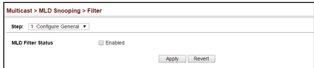
**Configuring MLD Filter Profiles** Use the Multicast > MLD Snooping > Filter (Configure Profile – Add) page to create an MLD profile and set its access mode. Then use the (Add Multicast Group Range) page to configure the multicast groups to filter.
