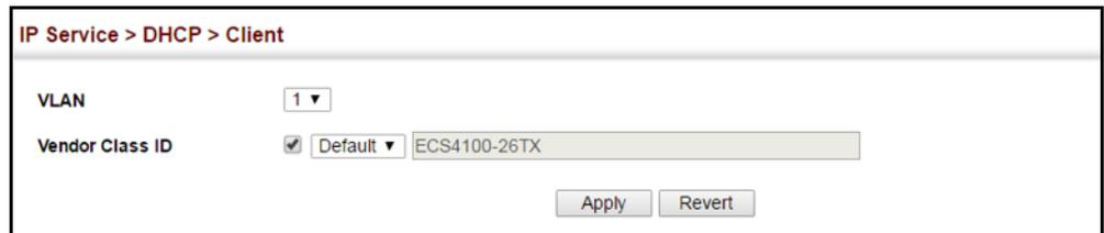
The screenshot shows a web interface for configuring DHCP Client settings. The breadcrumb path is "IP Service > DHCP > Client". There are two main configuration fields: "VLAN" with a dropdown menu showing "1", and "Vendor Class ID" which has a checked checkbox, a dropdown menu showing "Default", and a text input field containing "ECS4100-26TX". At the bottom right, there are "Apply" and "Revert" buttons.
