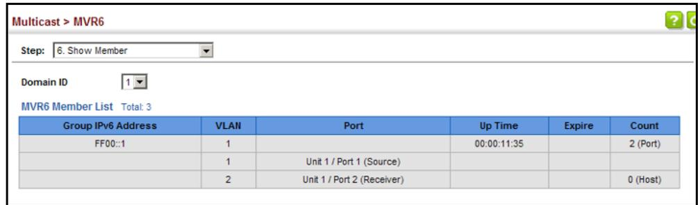
The screenshot shows the 'Multicast > MVR6' configuration page. At the top, there is a 'Step:' dropdown menu set to '6. Show Member'. Below that is a 'Domain ID' dropdown menu set to '1'. The main content is the 'MVR6 Member List' table, which has a 'Total: 3' indicator. The table has six columns: Group IPv6 Address, VLAN, Port, Up Time, Expire, and Count. The data rows are as follows:
