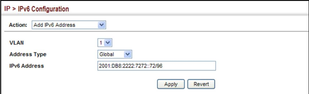
The screenshot shows the 'IP > IPv6 Configuration' web interface. The 'Action' dropdown is set to 'Add IPv6 Address'. The 'VLAN' dropdown is set to '1'. The 'Address Type' dropdown is set to 'Global'. The 'IPv6 Address' text field contains '2001:DB8:2222:7272::72/96'. There are 'Apply' and 'Revert' buttons at the bottom right.
