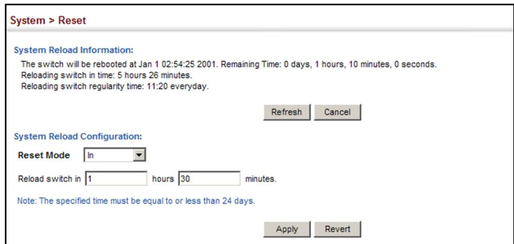
Figure 28: Restarting the Switch (At)
