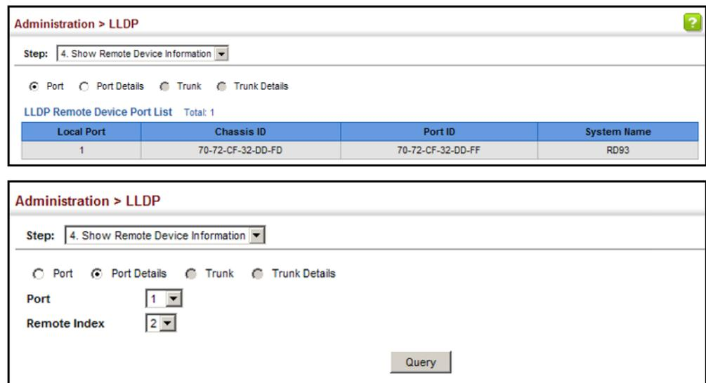
Figure 255: Displaying Remote Device Information for LLDP (Port Details)
