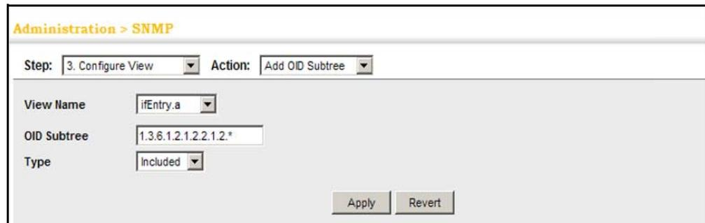
To show the OID branches configured for the SNMP views of the switch's MIB database:
