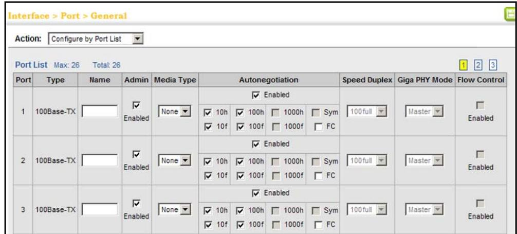
**CONFIGURING BY PORT RANGE** Use the Interface > Port > General (Configure by Port Range) page to enable/disable an interface, set auto-negotiation and the interface capabilities to advertise, or manually fix the speed, duplex mode, and flow control.
