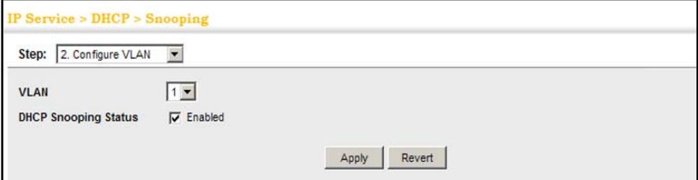
The screenshot shows a web interface for configuring DHCP Snooping. The breadcrumb path is "IP Service > DHCP > Snooping". The "Step" dropdown menu is set to "2. Configure VLAN". Below this, there is a "VLAN" dropdown menu set to "1". The "DHCP Snooping Status" is checked and labeled "Enabled". At the bottom right, there are two buttons: "Apply" and "Revert".
