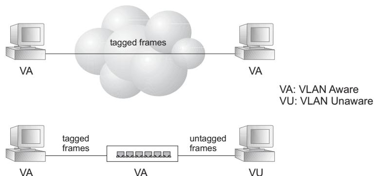
**VLAN Classification** – When the switch receives a frame, it classifies the frame in one of two ways. If the frame is untagged, the switch assigns the frame to an associated VLAN (based on the default VLAN ID of the
