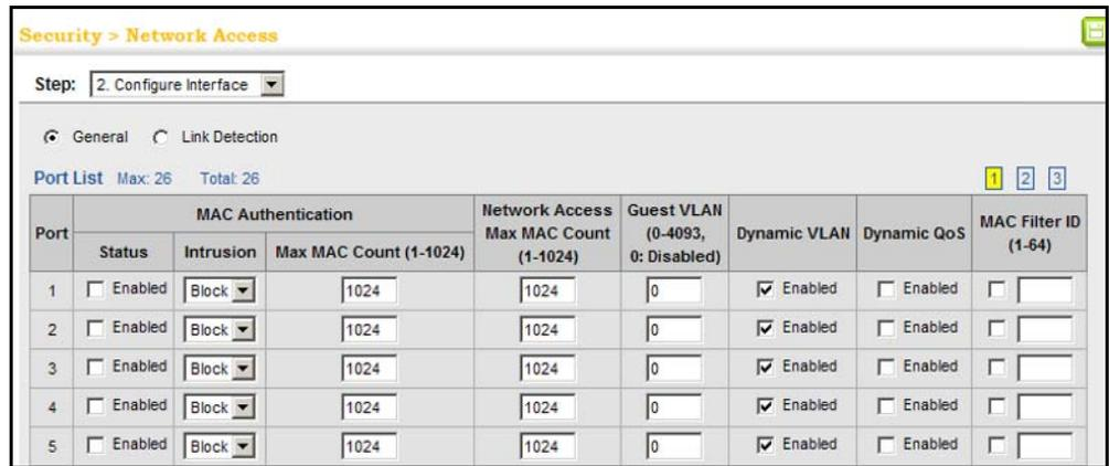
**CONFIGURING PORT LINK DETECTION** Use the Security > Network Access (Configure Interface - Link Detection) page to send an SNMP trap and/or shut down a port when a link event occurs.
