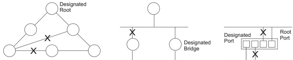
Once a stable network topology has been established, all bridges listen for Hello BPDUs (Bridge Protocol Data Units) transmitted from the Root Bridge. If a bridge does not get a Hello BPDU after a predefined interval (Maximum Age), the bridge assumes that the link to the Root Bridge is down. This bridge will then initiate negotiations with other bridges to reconfigure the network to reestablish a valid network topology.
