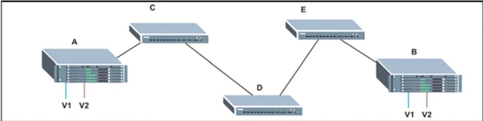
Without VLAN trunking, you would have to configure VLANs 1 and 2 on all intermediate switches – C, D and E; otherwise these switches would drop any frames with unknown VLAN group tags. However, by enabling VLAN trunking on the intermediate switch ports along the path connecting VLANs 1 and 2, you only need to create these VLAN groups
