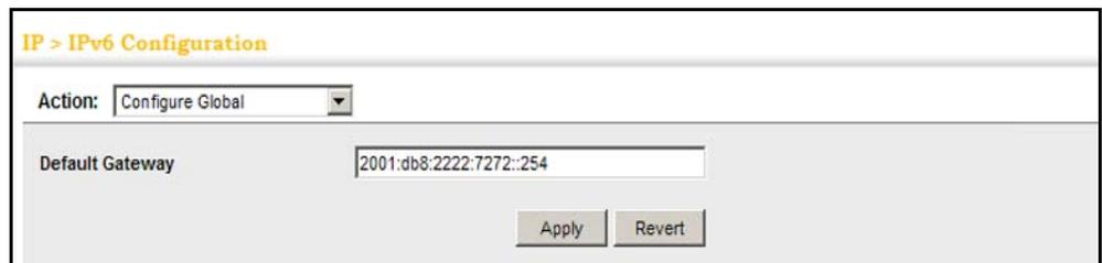
The screenshot shows a web interface titled "IP > IPv6 Configuration". At the top, there is a breadcrumb trail "IP > IPv6 Configuration". Below this, there is a section labeled "Action:" with a dropdown menu currently set to "Configure Global". Underneath, there is a field labeled "Default Gateway" with the value "2001:db8:2222:7272::254" entered. At the bottom right of the form, there are two buttons: "Apply" and "Revert".
