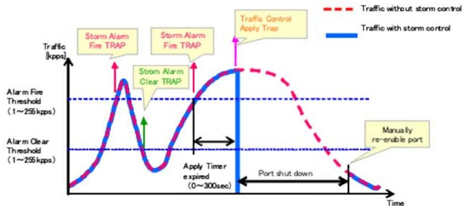
The key elements of this diagram are the same as that described in the preceding diagram, except that automatic release of the control response is not provided. When traffic control is applied, you must manually re-enable the port.
