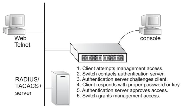
RADIUS uses UDP while TACACS+ uses TCP. UDP only offers best effort delivery, while TCP offers a more reliable connection-oriented transport. Also, note that RADIUS encrypts only the password in the access-request
