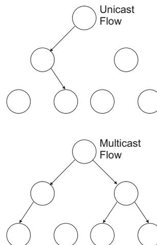
This switch can use Internet Group Management Protocol (IGMP) to filter multicast traffic. IGMP Snooping can be used to passively monitor or “snoop” on exchanges between attached hosts and an IGMP-enabled
