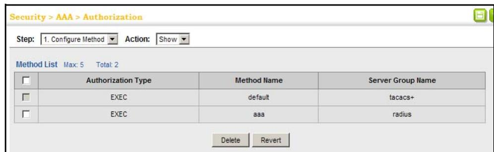
To configure the authorization method applied to local console, Telnet, or SSH connections:
