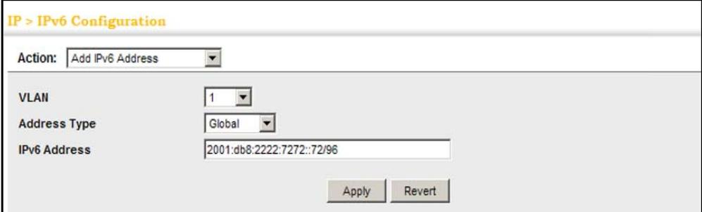
The screenshot shows the 'IP > IPv6 Configuration' web interface. At the top, there is a breadcrumb 'IP > IPv6 Configuration'. Below it, the 'Action' dropdown menu is set to 'Add IPv6 Address'. The 'VLAN' field is a dropdown menu with '1' selected. The 'Address Type' field is a dropdown menu with 'Global' selected. The 'IPv6 Address' field is a text input containing '2001:db8:2222:7272::72/96'. At the bottom right, there are two buttons: 'Apply' and 'Revert'.
