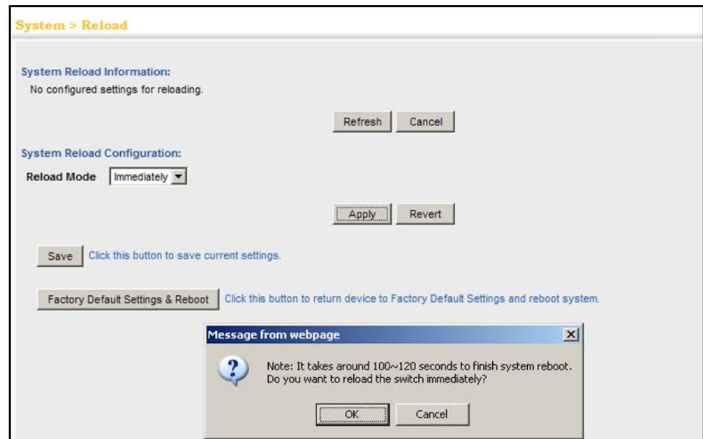
Figure 22: Restarting the Switch (In)
