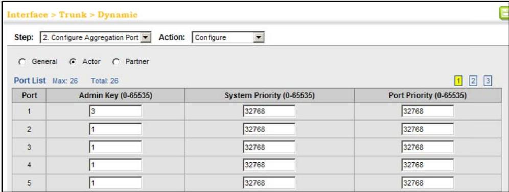
To configure the connection parameters for a dynamic trunk:
