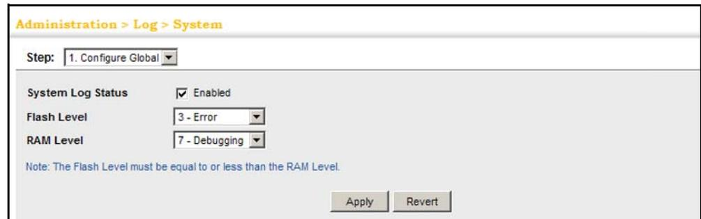
The screenshot shows a web interface for configuring system memory logs. The breadcrumb navigation is "Administration > Log > System". The "Step:" dropdown is set to "1. Configure Global". The "System Log Status" is checked and set to "Enabled". The "Flash Level" is set to "3 - Error" and the "RAM Level" is set to "7 - Debugging". A note below the levels states: "Note: The Flash Level must be equal to or less than the RAM Level." At the bottom right, there are "Apply" and "Revert" buttons.
