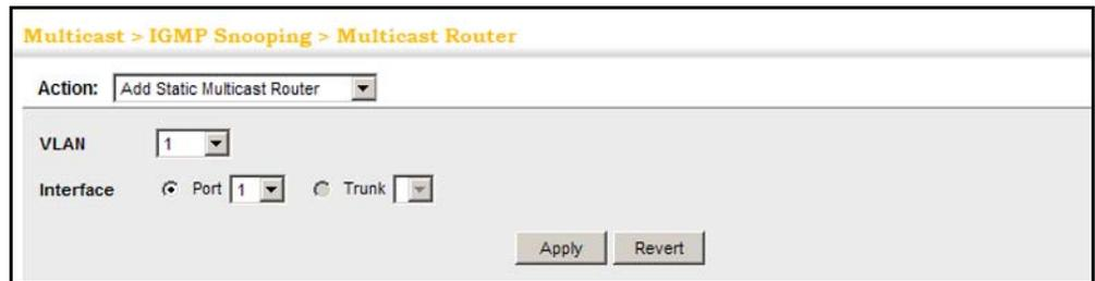
To show the static interfaces attached to a multicast router:
