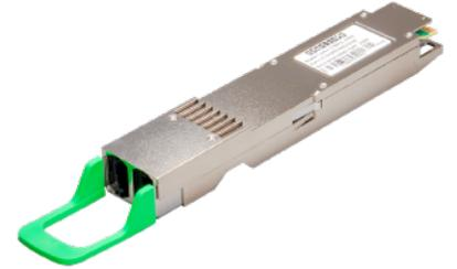
Based on a 5nm DSP and cooled 1310 EML laser technology, the ET8001-2DR4 is an 800G 2 x DR4 OSFP transceiver module compliant with the 800 Gigabit hot-pluggable OSFP Multi-Source Agreement (MSA) used for up to 8 x 100G PAM4 data rates over 500 m single mode fiber.
