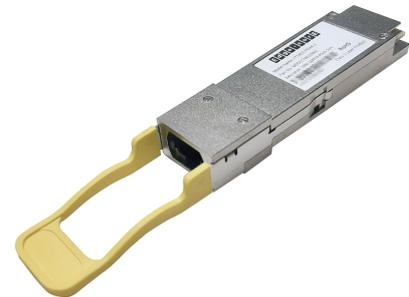
Edgecore’s ET7402-PSM2-2 QSFP28 transceiver modules are designed for use in 100 Gigabit Ethernet links of up to 2 km of single mode fiber. They are compliant with the QSFP28 MSA and portions of IEEE P802.3bm . Digital diagnostics functions are available via the I2C interface, as specified by the QSFP28 MSA. The QSFP28 full-duplex optical module offers 4 independent transmit and receive channels, each capable of 25Gb/s operation for an aggregate data rate of 100Gb/s.
