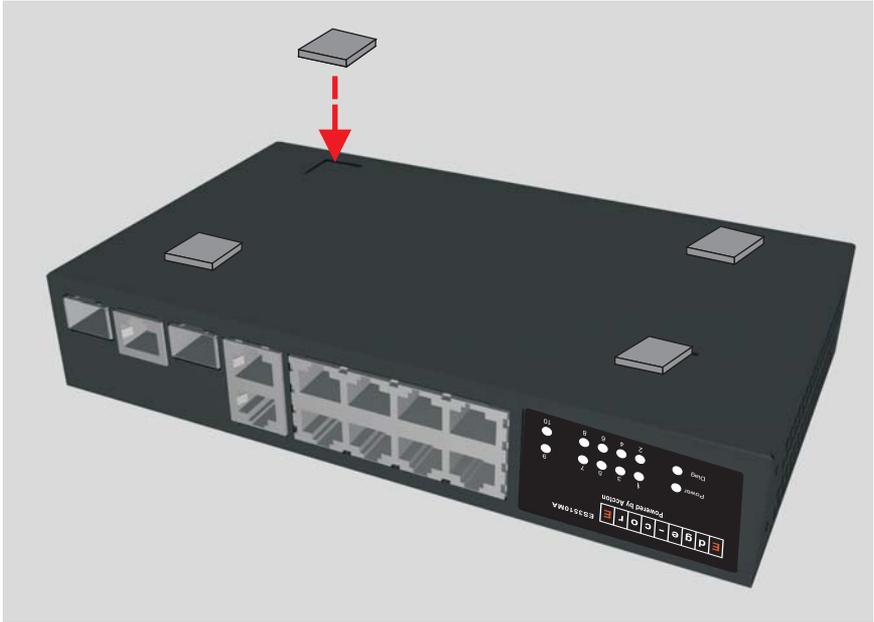
2. Set the device on a flat surface near an AC power source, making sure there are at least two inches of space on all sides for proper air flow.
