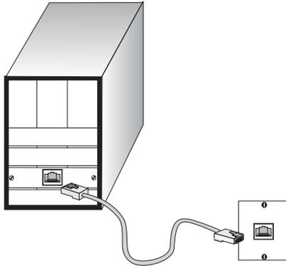
2. If the device is a network card and the switch is in the wiring closet, attach the other end of the cable segment to a modular wall outlet that is connected to the wiring closet. (See the section “[Fiber Optic SFP Devices](#).”) Otherwise, attach the other end to an available port on the switch.
