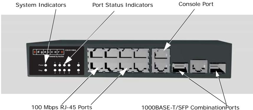
1. If an SFP transceiver is plugged in, the corresponding RJ-45 port is disabled for ports 9-10.
