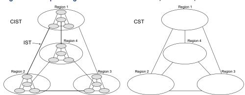
Figure 124: Spanning Tree – Common Internal, Common, Internal
