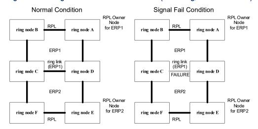
Figure 320: Ring Interconnection Architecture (Multi-ring/Ladder Network)
