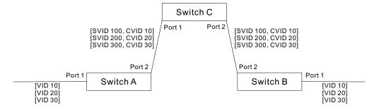
Step 1. Configure Switch A and B.
