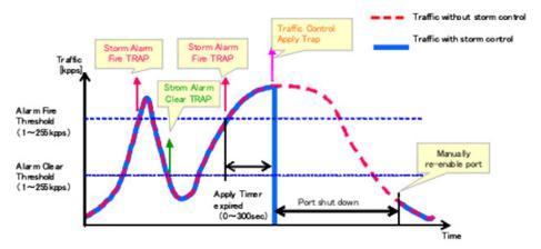
Figure 4: Storm Control by Shutting Down a Port
