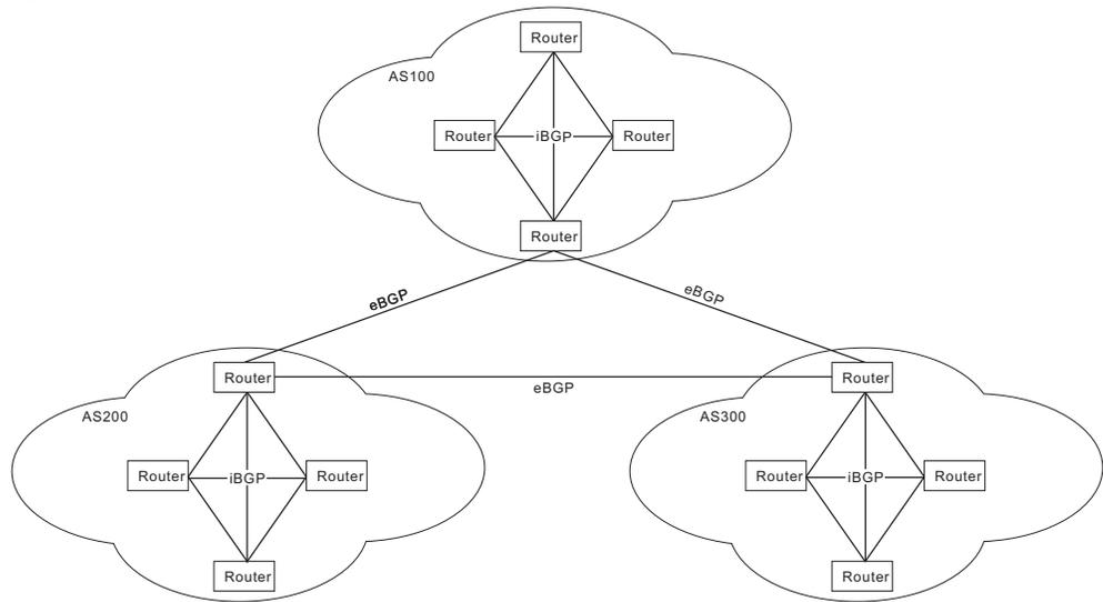
**External BGP** – eBGP interconnects different ASs through border routers, or eBGP peers. These peering routers are commonly connected over a WAN link using a single physical path. Alternatively, multiple eBGP peer connections may be used to provide redundancy or load balancing. Distinct BGP sessions are used between redundancy peers to ensure that if one session fails, another will take over.
