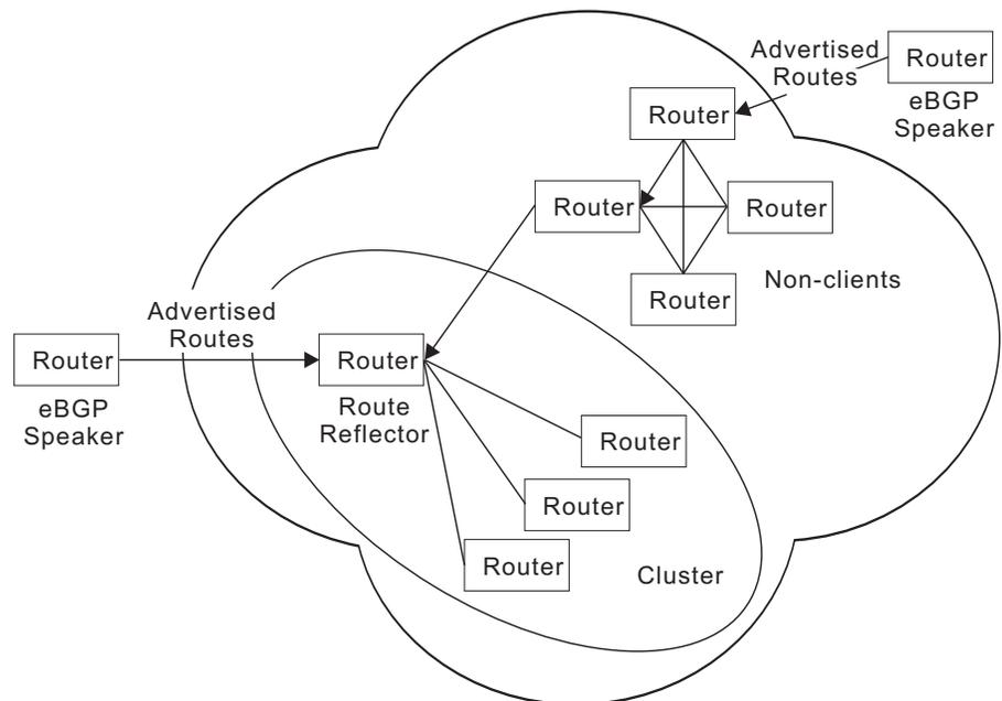
If there is only one route reflector in a cluster, that router would still have to process the same number of routing messages that would be required if it were in a fully meshed network. It is therefore preferable to use more than one route reflector in a cluster to reduce the overall number of iBGP sessions a single reflector has to handle.
