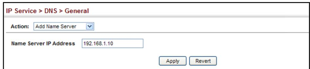
The screenshot shows a web interface for configuring DNS. At the top, the breadcrumb path is "IP Service > DNS > General". Below this, there is an "Action:" label followed by a dropdown menu currently set to "Add Name Server". Underneath, there is a "Name Server IP Address" label followed by a text input field containing the IP address "192.168.1.10". At the bottom right of the form, there are two buttons: "Apply" and "Revert".
