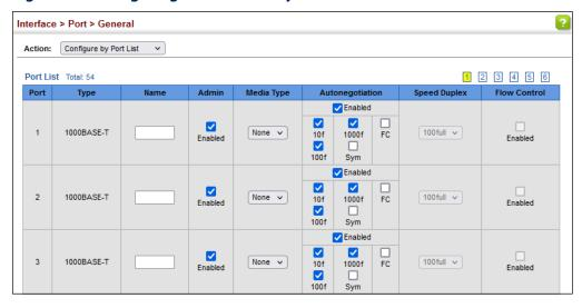
Configuring by Use the Interface > Port > General (Configure by Port Range) page to enable/ Port Range disable an interface or manually fix the speed, duplex mode, and flow control.
