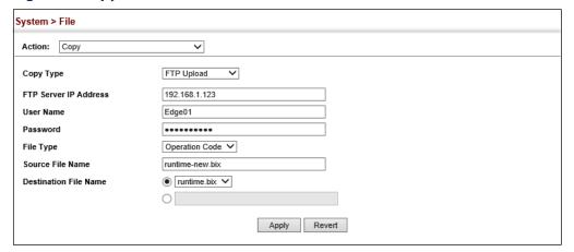
If you replaced a file currently used for startup and want to start using the new file, reboot the system via the System > Reset menu.
