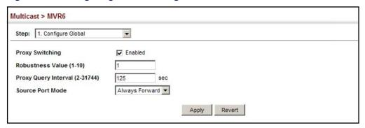
**Configuring MVR6** Use the Multicast > MVR6 (Configure Domain) page to enable MVR6 globally on the **Domain Settings** switch, and select the VLAN that will serve as the sole channel for common multicast streams supported by the service provider.
