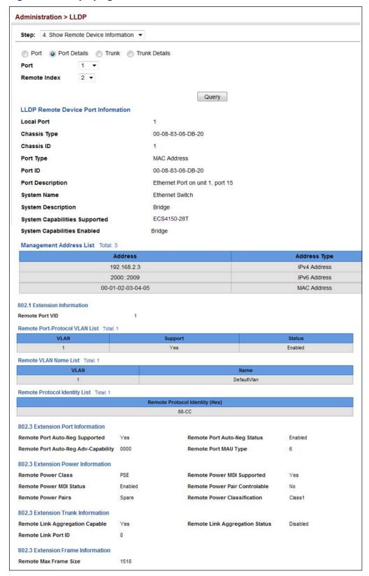
Additional information displayed by an end-point device which advertises LLDP-MED TLVs is shown in the following figure.
