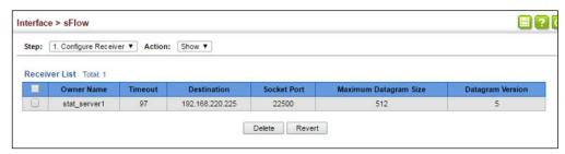
Configuring an sFlow Use the Interface > sFlow (Configure Details – Add) page to enable an sFlow polling Polling Instance data source that polls periodically based on a specified time interval, or an sFlow data source instance that takes samples periodically based on the number of packets processed.
