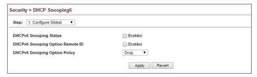
**DHCPv6 Snooping** Use the Security > DHCP Snooping6 (Configure VLAN) page to enable or disable **VLAN Configuration** DHCPv6 snooping on specific VLANs.
