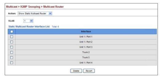
Multicast routers that are attached to ports on the switch use information obtained from IGMP, along with a multicast routing protocol (such as PIM) to support IP multicasting across the Internet. These routers may be dynamically discovered by the switch or statically assigned to an interface on the switch.
