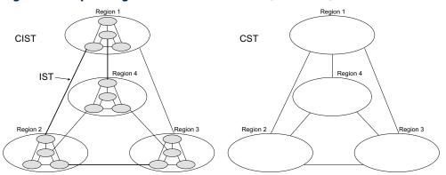
MSTP connects all bridges and LAN segments with a single Common and Internal Spanning Tree (CIST). The CIST is formed as a result of the running spanning tree algorithm between switches that support the STP, RSTP, MSTP protocols.
