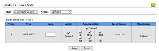
To display trunk connection parameters:
