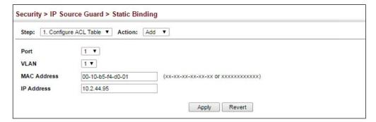
To display static bindings for IP Source Guard:
