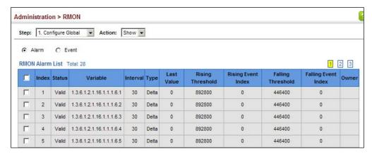
**Configuring RMON** Use the Administration > RMON (Configure Global - Add - Event) page to set the **Events** action to take when an alarm is triggered. The response can include logging the alarm or sending a message to a trap manager. Alarms and corresponding events provide a way of immediately responding to critical network problems.
