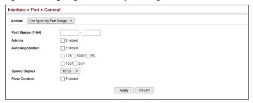
**Displaying** Use the Interface > Port > General (Show Information) page to display the current Connection Status connection status, including link state, speed/duplex mode, flow control, and autonegotiation.
