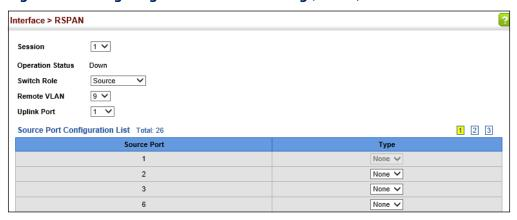
Figure 65: Configuring Remote Port Mirroring (Intermediate)
