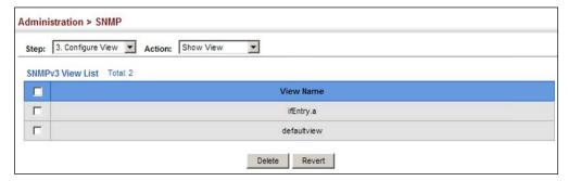
To add an object identifier to an existing SNMP view of the switch's MIB database:
