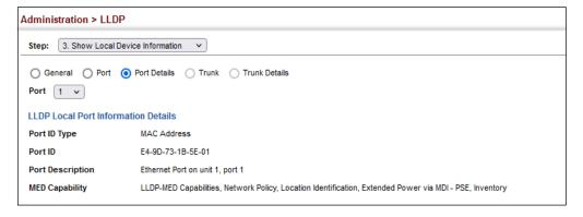
**Displaying LLDP** Use the Administration > LLDP (Show Remote Device Information) page to display Remote Device information about devices connected directly to the switch's ports which are **Information** advertising information through LLDP, or to display detailed information about an LLDP-enabled device connected to a specific port on the local switch.
