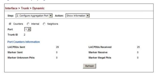
**Displaying LACP** Use the Interface > Trunk > Dynamic (Configure Aggregation Port - Show Settings and Status Information - Internal) page to display the configuration settings and operational for the Local Side state for the local side of a link aggregation.
