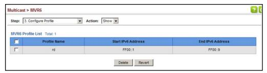
To assign an MVR6 group address profile to a domain:
