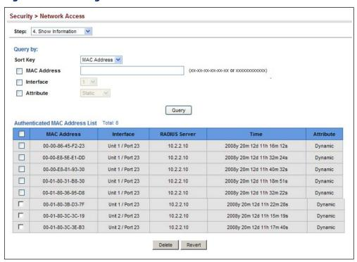
Figure 199: Showing Addresses Authenticated for Network Access
