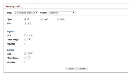
**Showing ACL** Use the Security > ACL > Configure Interface (Show Hardware Counters) page to Hardware Counters show statistics for ACL hardware counters.
