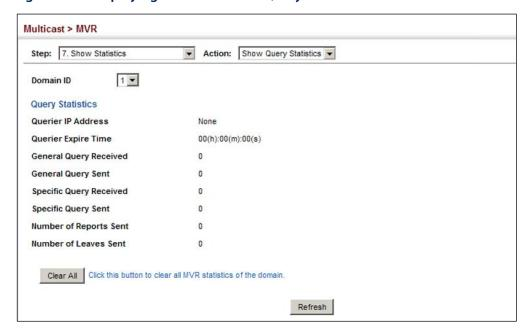
To display MVR protocol-related statistics for a VLAN, Port or Trunk:
