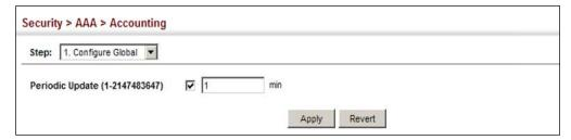
To configure the accounting method applied to various service types and the assigned server group:
