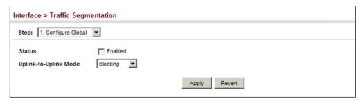
**Configuring Uplink** Use the Interface > Traffic Segmentation (Configure Session) page to assign the and Downlink Ports downlink and uplink ports to use in the segmented group. Ports designated as downlink ports can not communicate with any other ports on the switch except for the uplink ports. Uplink ports can communicate with any other ports on the switch and with any designated downlink ports.
