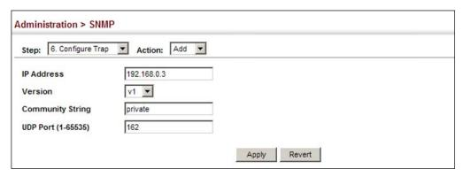
**Figure 293: Configuring Trap Managers** (SNMPv2c)
