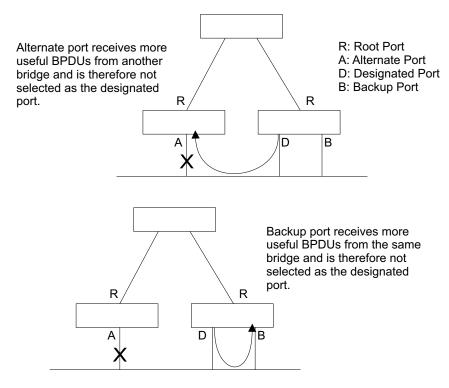
The criteria used for determining the port role is based on root bridge ID, root path cost, designated bridge, designated port, port priority, and port number, in that order and as applicable to the role under question.
