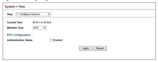
**Configuring** Use the System > Time (Configure Time Server) pages to specify the IP address for **Time Servers** NTP/SNTP time servers, or to set the authentication key for NTP time servers.
