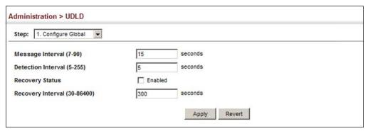
Configuring UDLD Use the Administration > UDLD (Configure Interface) page to enable UDLD and Interface Settings aggressive mode which reduces the shut-down delay after loss of bidirectional connectivity is detected.
