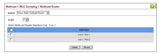
To show all the interfaces attached to a multicast router:
