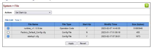
To start using the new firmware or configuration settings, reboot the system via the System > Reset menu.
