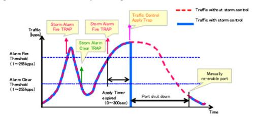
Figure 143: Storm Control by Shutting Down a Port
