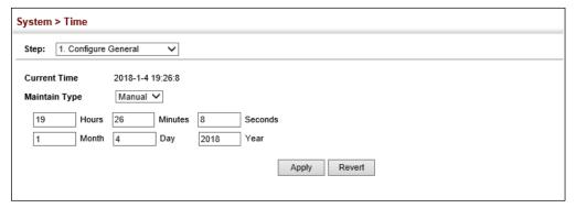
**Setting the SNTP** Use the System > Time (Configure General - SNTP) page to set the polling interval at **Polling Interval** which the switch will query the specified time servers.
