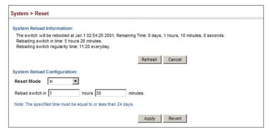
Figure 28: Restarting the Switch (At)
