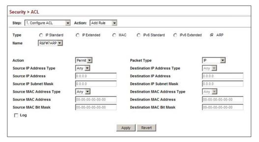
**Binding a Port to an** After configuring ACLs, use the Security > ACL (Configure Interface – Configure) Access Control List page to bind the ports that need to filter traffic to the appropriate ACLs.
