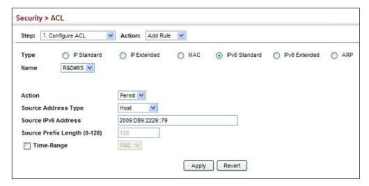
Configuring an Use the Security > ACL (Configure ACL - Add Rule - IPv6 Extended) page to **Extended IPv6 ACL** configure an Extended IPv6 ACL.
