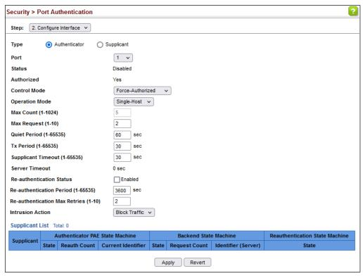
Figure 223: Configuring Interface Settings for 802.1X Port Authenticator
