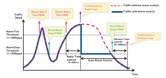
Figure 142: Storm Control by Limiting the Traffic Rate
