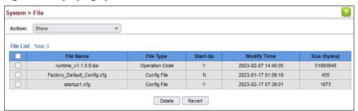
**Automatic Operation** Use the System > File (Automatic Operation Code Upgrade) page to automatically Code Upgrade download an operation code file when a file newer than the currently installed one is discovered on the file server. After the file is transferred from the server and successfully written to the file system, it is automatically set as the startup file, and the switch is rebooted.
