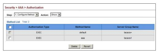
To configure the authorization method applied to local console, Telnet, or SSH connections:
