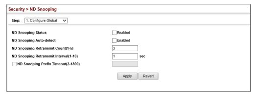
ND Snooping VLAN Use the Security > ND Snooping > Configure VLAN (Add) page to enable ND **Configuration** Snooping on a specified VLAN or range of VLANs.
