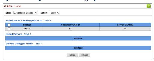
The preceding example sets the SVID to 44 in the outer tag for egress packets exiting port 6 when the packet's CVID is 55. For a more detailed example, see the "switchport dot1q-tunnel service match cvid" command in the CLI Reference Guide.
