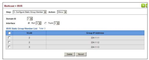
**Displaying MVR** Use the Multicast > MVR (Show Member) page to show the multicast groups either **Receiver Groups** statically or dynamically assigned to the MVR receiver groups on each interface.
