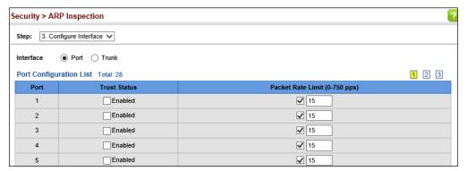
**Displaying** Use the Security > ARP Inspection (Show Information - Show Statistics) page to **ARP Inspection** display statistics about the number of ARP packets processed, or dropped for **Statistics** various reasons.
