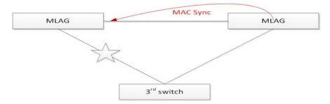
When the MLAG peer member is down or nonexistent, learned MAC addresses are synced through the peer link for the MLAG will be removed automatically.
