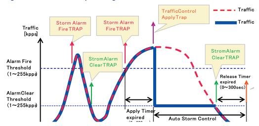
Figure 3: Storm Control by Limiting the Traffic Rate
