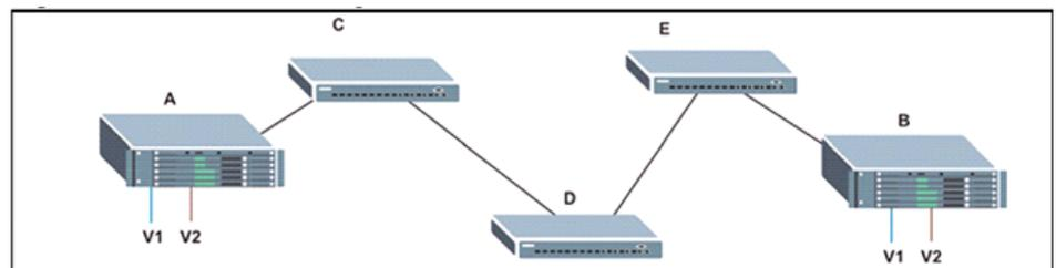
Without VLAN trunking, you would have to configure VLANs 1 and 2 on all intermediate switches – C, D and E; otherwise these switches would drop any frames with unknown VLAN group tags. However, by enabling VLAN trunking on the intermediate switch ports along the path connecting VLANs 1 and 2, you only need to create these VLAN groups in switches A and B. Switches C, D
