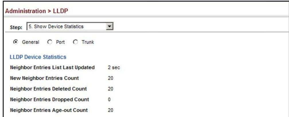
**Figure 254: Displaying LLDP Device Statistics (Port)**
