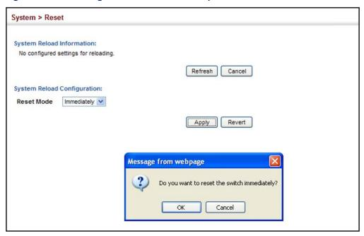
Figure 30: Restarting the Switch (In)
