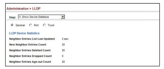
Figure 273: Displaying LLDP Device Statistics (Port)
