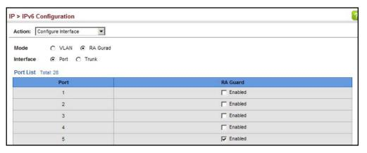
Figure 451: Configuring RA Guard for an IPv6 Interface
