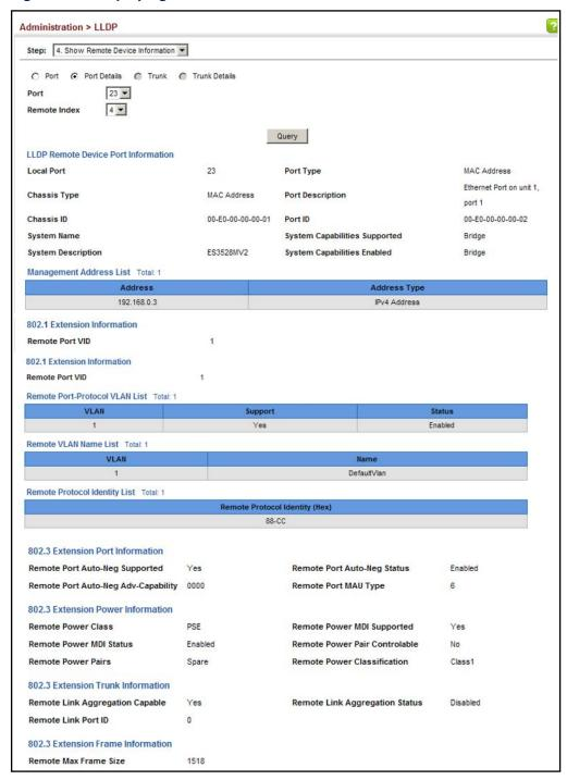
Figure 270: Displaying Remote Device Information for LLDP (Trunk)
