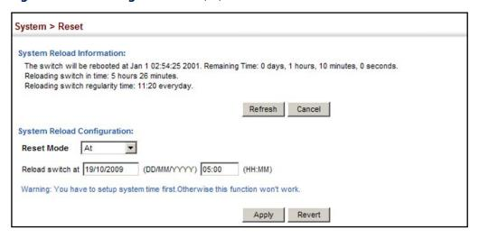
Figure 32: Restarting the Switch (Regularly)
