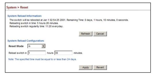
Figure 31: Restarting the Switch (At)
