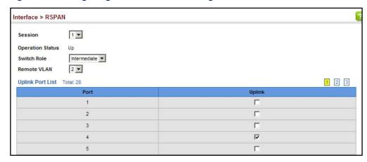
Figure 69: Configuring Remote Port Mirroring (Destination)
