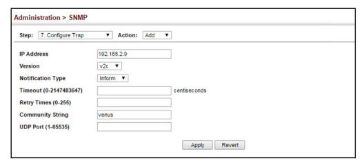
Figure 294: Configuring Trap Managers (SNMPv3)
