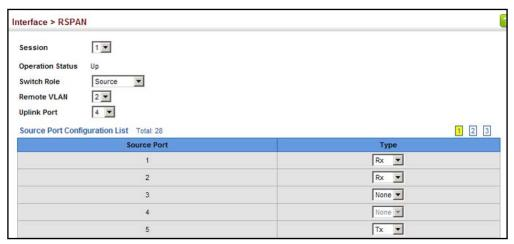
Figure 68: Configuring Remote Port Mirroring (Intermediate)
