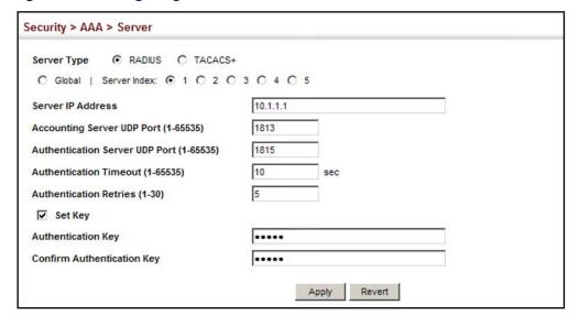
Figure 178: Configuring Remote Authentication Server (TACACS+)
