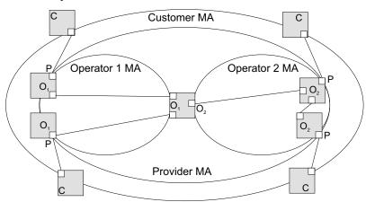
**Figure 337: Multiple CFM Maintenance Domains**
