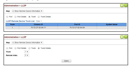
Figure 271: Displaying Remote Device Information for LLDP (Trunk Details)<sup>16</sup>
