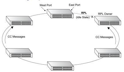
**Figure 320: ERPS Ring Components**
