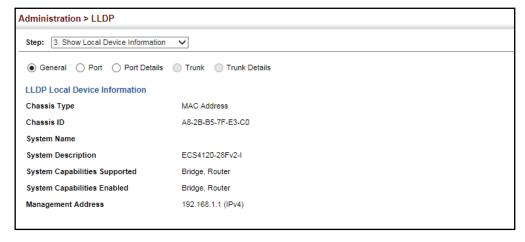
Figure 264: Displaying Local Device Information for LLDP (Port)
