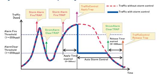
Figure 139: Storm Control by Limiting the Traffic Rate
