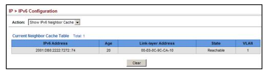
**Showing** Use the IP > IPv6 Configuration (Show Statistics) page to display statistics about **IPv6 Statistics** IPv6 traffic passing through this switch.
