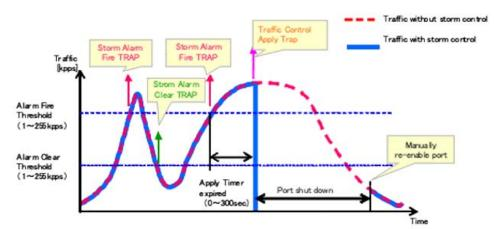
Figure 140: Storm Control by Shutting Down a Port
