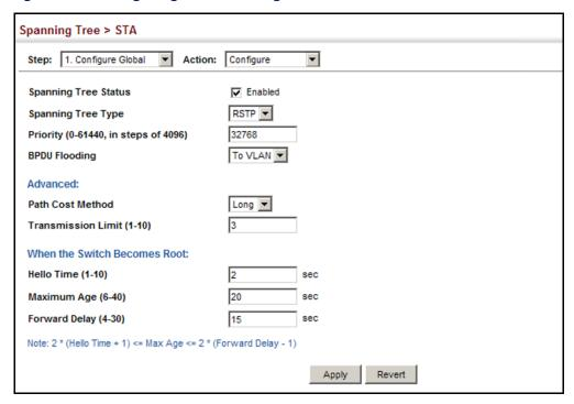
Figure 123: Configuring Global Settings for STA (MSTP)
