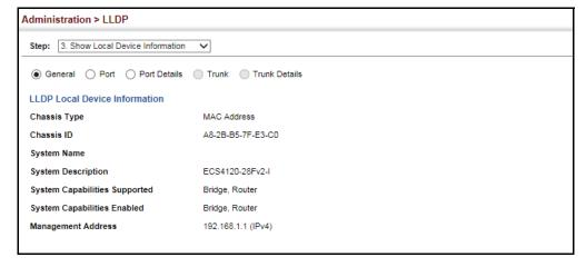
Figure 264: Displaying Local Device Information for LLDP (Port)
