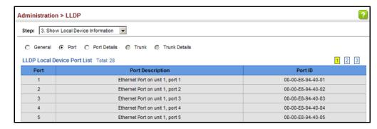
Figure 265: Displaying Local Device Information for LLDP (Port Details)
