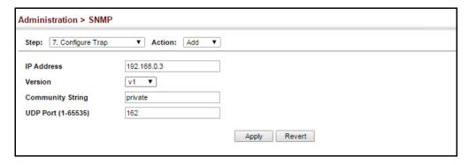
Figure 293: Configuring Trap Managers (SNMPv2c)
