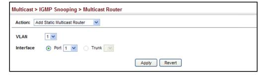
To show the static interfaces attached to a multicast router:
