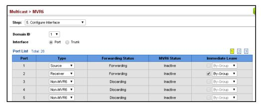
Assigning Static Use the Multicast > MVR6 (Configure Static Group Member) page to statically bind MVR6 Multicast multicast groups to a port which will receive long-term multicast streams **Groups to Interfaces** associated with a stable set of hosts.
