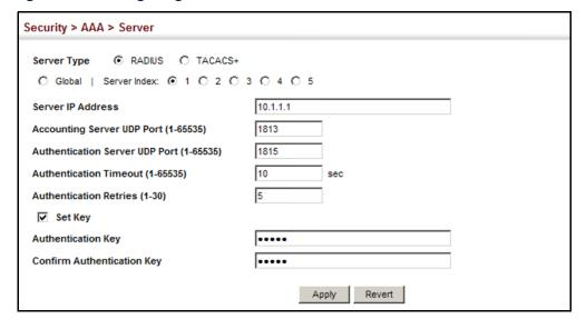
Figure 178: Configuring Remote Authentication Server (TACACS+)
