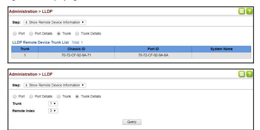
Figure 271: Displaying Remote Device Information for LLDP (Trunk Details)<sup>16</sup>
