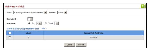
**Displaying MVR6** Use the Multicast > MVR6 (Show Member) page to show the multicast groups **Receiver Groups** either statically or dynamically assigned to the MVR6 receiver groups on each interface.
