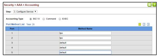
Figure 185: Configuring AAA Accounting Service for Command 0 to 15
