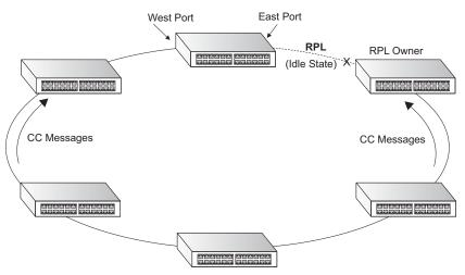
**Figure 320: ERPS Ring Components**
