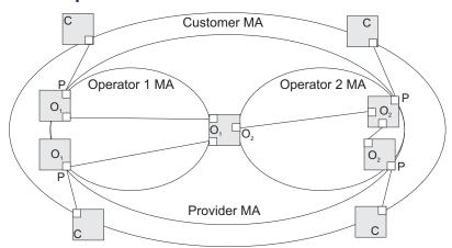
**Figure 337: Multiple CFM Maintenance Domains**
