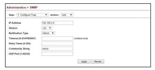
Figure 294: Configuring Trap Managers (SNMPv3)
