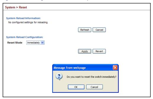
Figure 30: Restarting the Switch (In)
