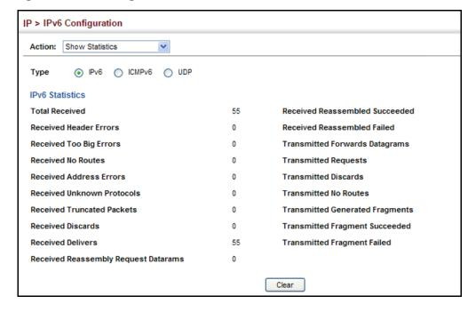
Figure 456: Showing IPv6 Statistics (ICMPv6)
