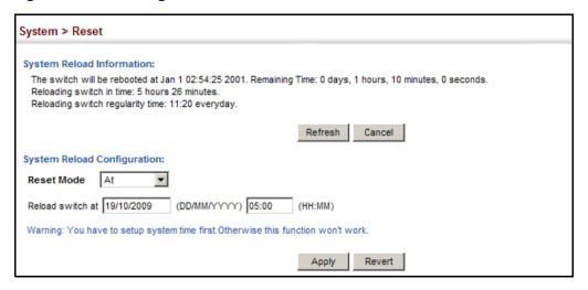
Figure 32: Restarting the Switch (Regularly)
