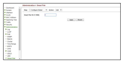
**Configuring Smart** Use the Administration > Smart Pair (Configure Smart Pair Global) to add the port Pair Interface Settings members of a Smart Pair. The ports must have spanning tree turned off to be available for selection.
