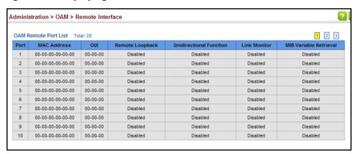
**Configuring a Remote** Use the Administration > OAM > Remote Loopback (Remote Loopback Test) page **Loopback Test** to initiate a loop back test to the peer device attached to the selected port.
