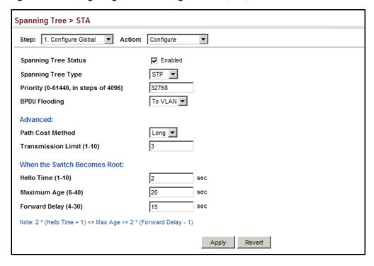
Figure 122: Configuring Global Settings for STA (RSTP)
