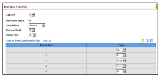
**Figure 68: Configuring Remote Port Mirroring (Intermediate)**
