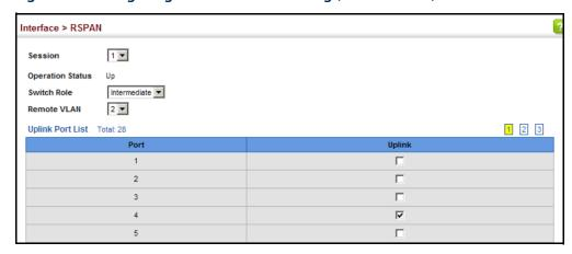
Figure 69: Configuring Remote Port Mirroring (Destination)
