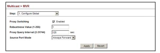
**Configuring MVR** Use the Multicast > MVR (Configure Domain) page to enable MVR globally on the **Domain Settings** switch, and select the VLAN that will serve as the sole channel for common multicast streams supported by the service provider.
