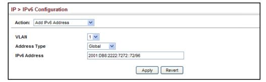
**Showing IPv6** Use the IP > IPv6 Configuration (Show IPv6 Address) page to display the IPv6 Addresses addresses assigned to an interface.
