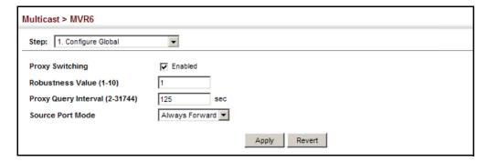
Configuring MVR6 Use the Multicast > MVR6 (Configure Domain) page to enable MVR6 globally on the **Domain Settings** switch, and select the VLAN that will serve as the sole channel for common multicast streams supported by the service provider.
