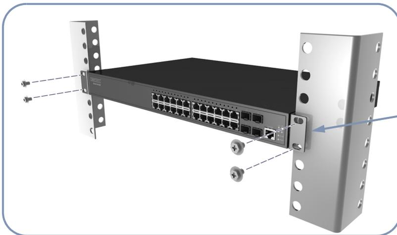
Attach the brackets to the switch, then use the rack mounting screws supplied with the rack to secure the switch in the rack.
