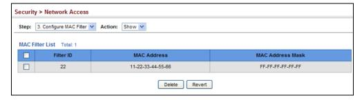
**Displaying Secure** Use the Security > Network Access (Show Information) page to display the MAC Address authenticated MAC addresses stored in the secure MAC address table. Information **Information** on the secure MAC entries can be displayed and selected entries can be removed from the table.
