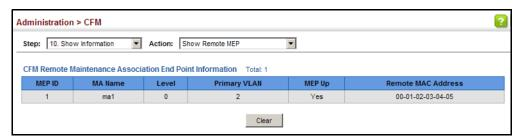
**Displaying Details for** Use the Administration > CFM > Show Information (Show Remote MEP Details) **Remote MEPs** page to show detailed information for MEPs located on other devices which have been discovered through continuity check messages, or statically configured in the MEP database and verified through cross-check messages.
