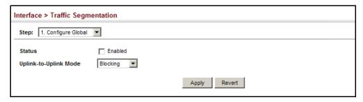
**Configuring Uplink** Use the Interface > Traffic Segmentation (Configure Session) page to assign the and Downlink Ports downlink and uplink ports to use in the segmented group. Ports designated as downlink ports can not communicate with any other ports on the switch except for the uplink ports. Uplink ports can communicate with any other ports on the switch and with any designated downlink ports.
