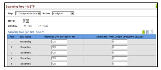
To display MSTP parameters for a port or trunk:
