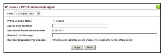
Configuring PPPoE IA Use the IP Service > PPPoE Intermediate Agent (Configure Interface) page to enable Interface Settings PPPoE IA on an interface, set trust status, enable vendor tag stripping, and set the circuit ID and remote ID.
