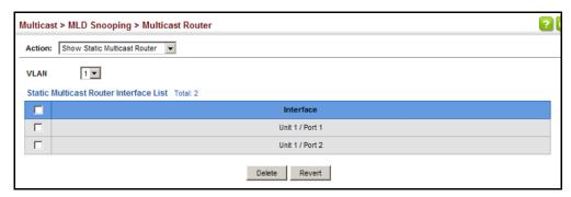
To show all the interfaces attached to a multicast router:
