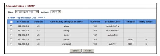
**Creating SNMP** Use the Administration > SNMP (Configure Notify Filter - Add) page to create an Notification Logs SNMP notification log.
