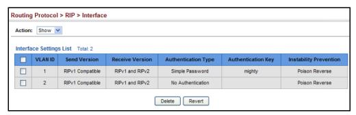
Displaying RIP Use the Routing Protocol > RIP > Statistics (Show Interface Information) page to Interface Settings display information about RIP interface configuration settings.
