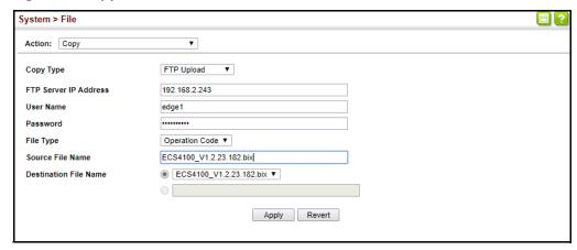
If you replaced a file currently used for startup and want to start using the new file, reboot the system via the System > Reset menu.
