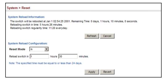
Figure 28: Restarting the Switch (At)
