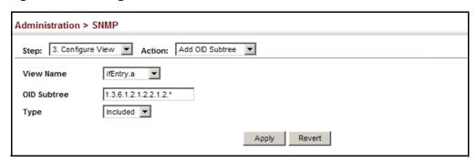
To show the OID branches configured for the SNMP views of the switch's MIB database:
