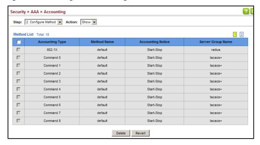
To configure the accounting method applied to specific interfaces, console commands entered at specific privilege levels, and local console, Telnet, or SSH connections:
