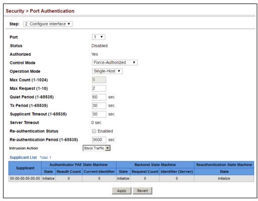
Figure 214: Configuring Interface Settings for 802.1X Port Authenticator
