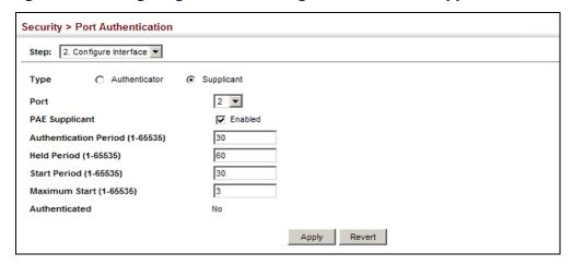
**Displaying** Use the Security > Port Authentication (Show Statistics) page to display statistics for **802.1X Statistics** dot1x protocol exchanges for any port.
