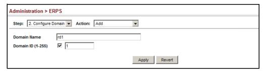
To configure the ERPS parameters for a ring:
