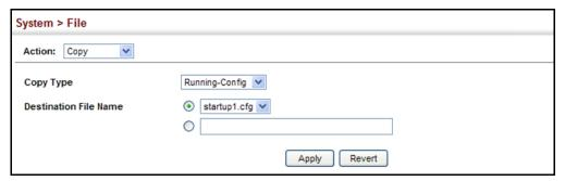
If you replaced a file currently used for startup and want to start using the new file, reboot the system via the System > Reset menu.
