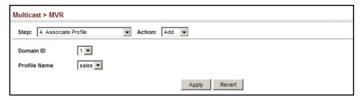
To show the MVR group address profiles assigned to a domain:
