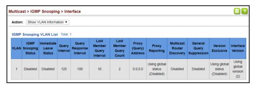
Filtering IGMP Packets Use the Multicast > IGMP Snooping > Interface (Configure Interface) page to on an Interface configure an interface to drop IGMP query packets or multicast data packets, or enable IGMP authentication.
