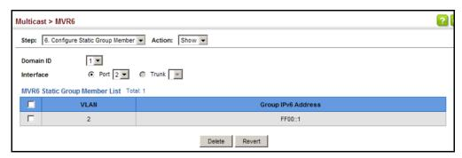
**Displaying MVR6** Use the Multicast > MVR6 (Show Member) page to show the multicast groups Receiver Groups either statically or dynamically assigned to the MVR6 receiver groups on each interface.
