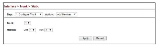
To configure connection parameters for a static trunk:
