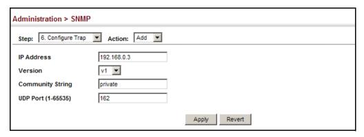
**Figure 279: Configuring Trap Managers** (SNMPv2c)
