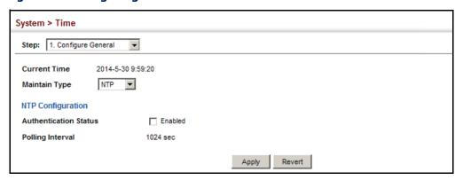
**Configuring** Use the System > Time (Configure Time Server) pages to specify the IP address for **Time Servers** NTP/SNTP time servers, or to set the authentication key for NTP time servers.
