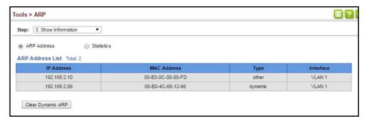
**Displaying** Use the Tools > ARP (Show Information) page to display statistics for ARP messages **ARP Statistics** crossing all interfaces on this switch.
