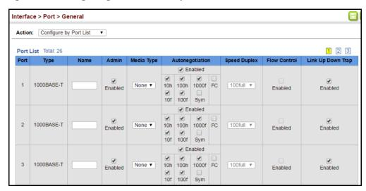
Configuring by Use the Interface > Port > General (Configure by Port Range) page to enable/ Port Range disable an interface, set auto-negotiation and the interface capabilities to advertise, or manually fix the speed, duplex mode, and flow control.
