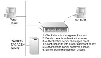
RADIUS uses UDP while TACACS+ uses TCP. UDP only offers best effort delivery, while TCP offers a more reliable connection-oriented transport. Also, note that
