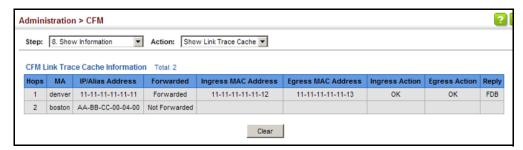
Displaying Fault Use the Administration > CFM > Show Information (Show Fault Notification Notification Settings Generator) page to display configuration settings for the fault notification generator.
