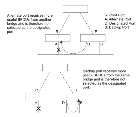
The criteria used for determining the port role is based on root bridge ID, root path cost, designated bridge, designated port, port priority, and port number, in that order and as applicable to the role under question.
