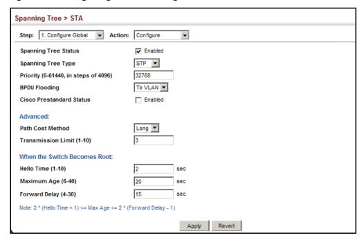
**Figure 99: Configuring Global Settings for STA** (RSTP)
