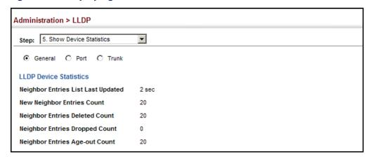
Figure 215: Displaying LLDP Device Statistics (Port)
