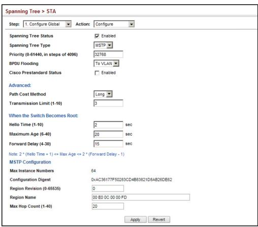
**Figure 100: Configuring Global Settings for STA** (MSTP)
