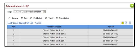
Figure 211: Displaying Local Device Information for LLDP (Port Details)
