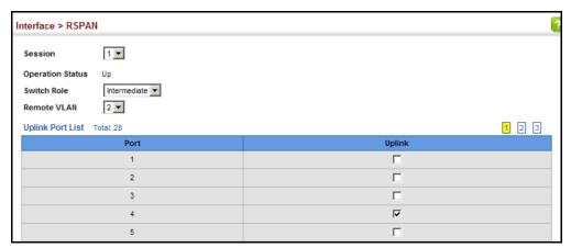
**Figure 64: Configuring Remote Port Mirroring (Destination)**
