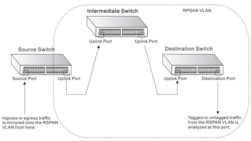
**Figure 61: Configuring Remote Port Mirroring**
