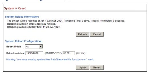
Figure 30: Restarting the Switch (Regularly)
