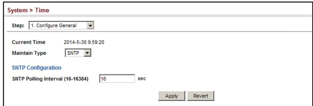
The screenshot shows a web interface for configuring system time. At the top, it says "System > Time". Below that, there is a "Step:" dropdown menu set to "1. Configure General". The "Current Time" is displayed as "2014-5-30 9:59:20". The "Maintain Type" is set to "SNTP" in a dropdown menu. Under the "SNTP Configuration" section, the "SNTP Polling Interval (16-16384)" is set to "16" seconds. At the bottom right, there are "Apply" and "Revert" buttons.
