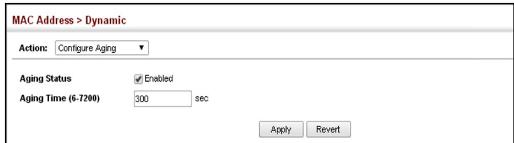
The screenshot shows a configuration page titled "MAC Address > Dynamic". At the top, there is a dropdown menu for "Action" set to "Configure Aging". Below this, the "Aging Status" is checked and labeled "Enabled". The "Aging Time (6-7200)" is set to "300" with the unit "sec" to its right. At the bottom right of the form, there are two buttons: "Apply" and "Revert".
