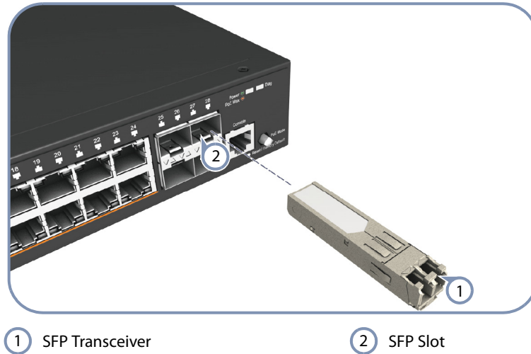
Figure 20: Inserting an SFP/SFP+ Transceiver into a Slot
