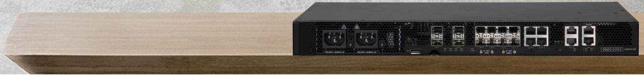
The Edgecore AS5915-16X is a compact-sized open cell site gateway platform that provides a combination of 1GE and 10 GE interfaces utilizing merchant silicon and an x86 processor to optimize performance for mobile networks.
