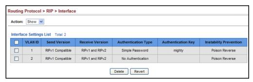
**Displaying RIP** Use the Routing Protocol > RIP > Statistics (Show Interface Information) page to Interface Settings display information about RIP interface configuration settings.
