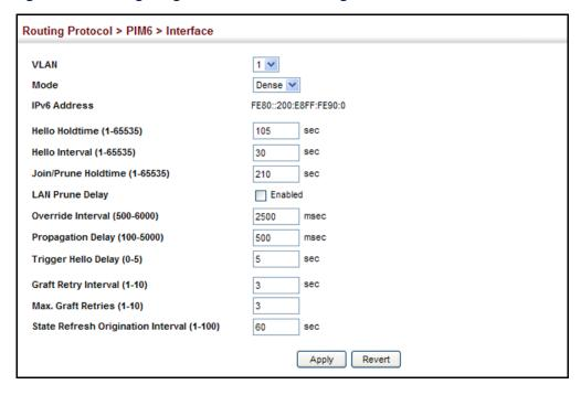
Figure 428: Configuring PIMv6 Interface Settings (Sparse Mode)
