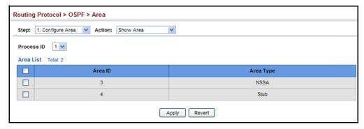
**Configuring NSSA** Use the Routing Protocol > OSPF > Area (Configure Area – Configure NSSA Area) **Settings** page to configure protocol settings for a not-so-stubby area (NSSA).
