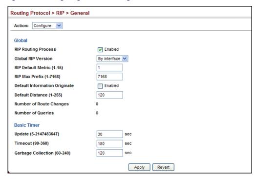
Clearing Entries from Use the Routing Protocol > RIP > General (Clear Route) page to clear entries from the Routing Table the routing table based on route type or a specific network address.
