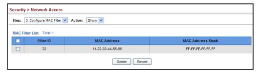
**Displaying Secure** Use the Security > Network Access (Show Information) page to display the MAC Address authenticated MAC addresses stored in the secure MAC address table. Information Information on the secure MAC entries can be displayed and selected entries can be removed from the table.
