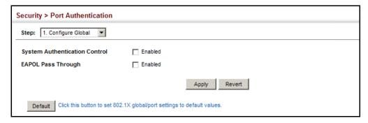
**Configuring Port** Use the Security > Port Authentication (Configure Interface) page to configure **Authenticator** 802.1X port settings for the switch as the local authenticator. When 802.1X is Settings for 802.1X enabled, you need to configure the parameters for the authentication process that runs between the client and the switch (i.e., authenticator), as well as the client identity lookup process that runs between the switch and authentication server.
