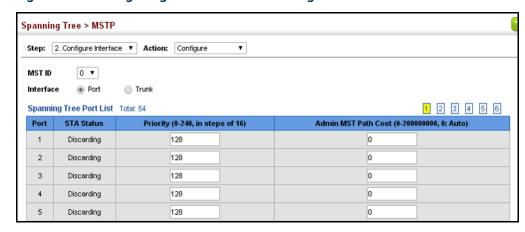
To display MSTP parameters for a port or trunk:
