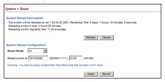
Figure 28: Restarting the Switch (Regularly)
