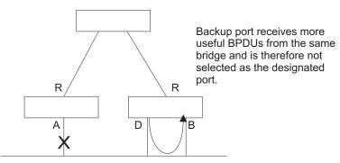
The criteria used for determining the port role is based on root bridge ID, root path cost, designated bridge, designated port, port priority, and port number, in that order and as applicable to the role under question.
