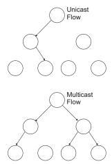
This switch can use Internet Group Management Protocol (IGMP) to filter multicast traffic. IGMP Snooping can be used to passively monitor or "snoop" on exchanges between attached hosts and an IGMP-enabled device, most commonly a multicast
