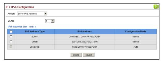
**Showing the IPv6** Use the IP > IPv6 Configuration (Show IPv6 Neighbor Cache) page to display the Neighbor Cache IPv6 addresses detected for neighbor devices.
