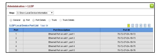
Figure 202: Displaying Local Device Information for LLDP (Port Details)
