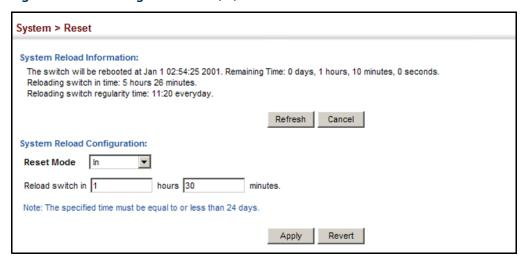
Figure 27: Restarting the Switch (At)
