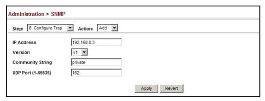
Figure 226: Configuring Trap Managers (SNMPv2c)
