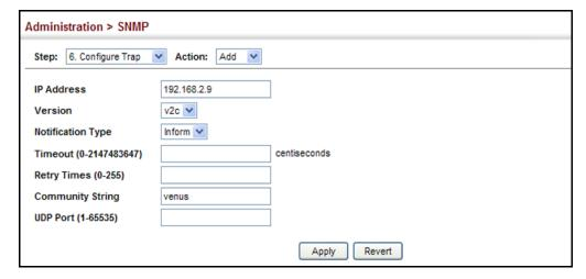
Figure 227: Configuring Trap Managers (SNMPv3)
