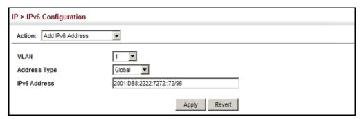
**Showing IPv6** Use the IP > IPv6 Configuration (Show IPv6 Address) page to display the IPv6 Addresses addresses assigned to an interface.
