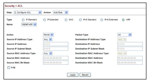
**Binding a Port to an** After configuring ACLs, use the Security > ACL (Configure Interface – Configure) Access Control List page to bind the ports that need to filter traffic to the appropriate ACLs. Only one access list (IPv4, IPv6 or MAC) can be assigned to an ingress or egress port.
