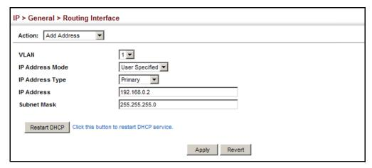
To obtain an dynamic IPv4 address through DHCP/BOOTP for the switch:
