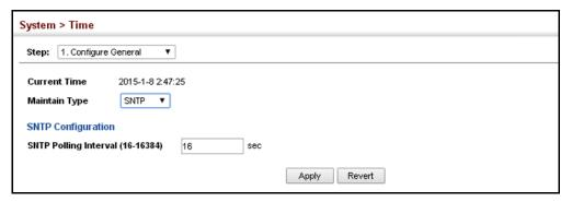
**Configuring NTP** Use the System > Time (Configure General - NTP) page to configure NTP authentication and show the polling interval at which the switch will query the specified time servers.
