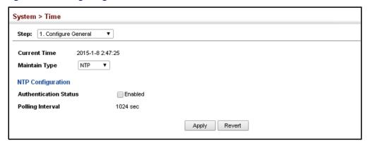
**Configuring Time** Use the System > Time (Configure Time Server) pages to specify the IP address for **Servers** NTP/SNTP time servers, or to set the authentication key for NTP time servers.
