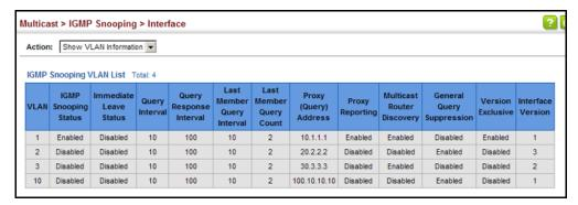
**Filtering IGMP Query** Use the Multicast > IGMP Snooping > Interface (Configure Interface) page to Packets configure an interface to drop IGMP guery packets.
