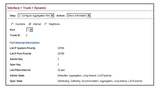
**Displaying LACP** Use the Interface > Trunk > Dynamic (Configure Aggregation Port - Show Settings and Status for Information - Neighbors) page to display the configuration settings and the Remote Side operational state for the remote side of a link aggregation.
