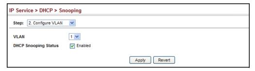
**Configuring Interfaces** Use the IP Service > DHCP > Snooping (Configure Interface) page to configure for DHCP Snooping switch interfaces as trusted or untrusted.
