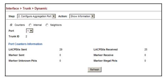
**Displaying LACP** Use the Interface > Trunk > Dynamic (Configure Aggregation Port - Show Settings and Status for Information - Internal) page to display the configuration settings and operational the Local Side state for the local side of a link aggregation.
