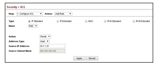
**Configuring an** Use the Security > ACL (Configure ACL - Add Rule - IP Extended) page to configure Extended IPv4 ACL an Extended IPv4 ACL.
