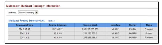
To display detailed information on a specific flow in multicast routing table:
