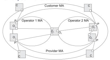
Note that the Service Instances within each domain shown above are based on a unique maintenance association for the specific users, distinguished by the domain name, maintenance level, maintenance association's name, and assigned VLAN.
