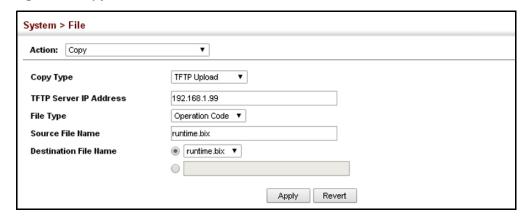
If you replaced a file currently used for startup and want to start using the new file, reboot the system via the System > Reset menu.
