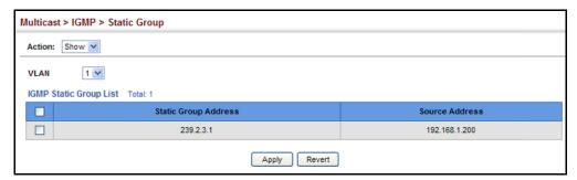
**Displaying Multicast** When IGMP (Layer 3) is enabled on the switch, use the Multicast > IGMP > Group **Group Information** Information pages to display the current multicast groups learned through IGMP. When IGMP (Layer 3) is disabled and IGMP (Layer 2) is enabled, the active multicast groups can be viewed on the Multicast > IGMP Snooping > Forwarding Entry page (see page 452).
