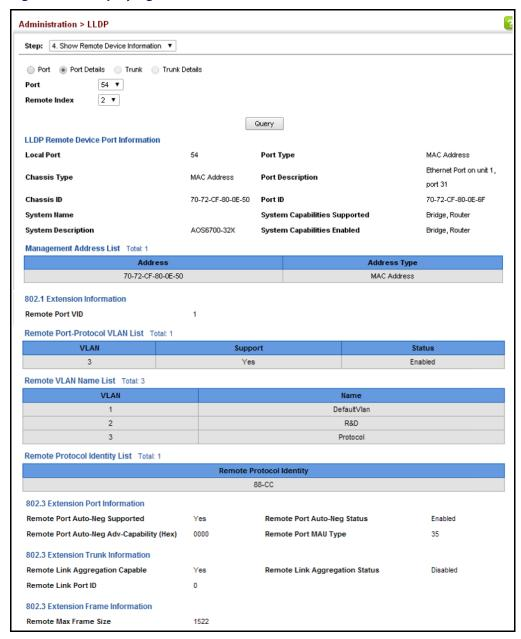
Additional information displayed by an end-point device which advertises LLDP-MED TLVs is shown in the following figure.
