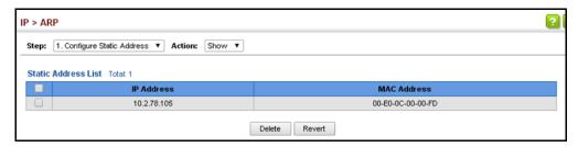
**Displaying Dynamic or** The ARP cache contains static entries, and entries for local interfaces, including Local ARP Entries subnet, host, and broadcast addresses. However, most entries will be dynamically learned through replies to broadcast messages. Use the IP > ARP (Show Information) page to display dynamic or local entries in the ARP cache.
