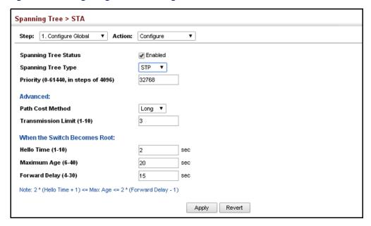
Figure 91: Configuring Global Settings for STA (RSTP)
