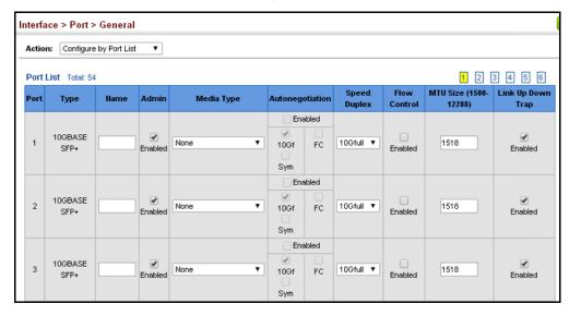
Configuring by Port Use the Interface > Port > General (Configure by Port Range) page to enable/ disable an interface, set auto-negotiation and the interface capabilities to advertise, or manually fix the speed, duplex mode, and flow control.
