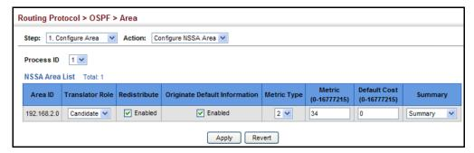
**Configuring Stub** Use the Routing Protocol > OSPF > Area (Configure Area – Configure Stub Area) **Settings** page to configure protocol settings for a stub.
