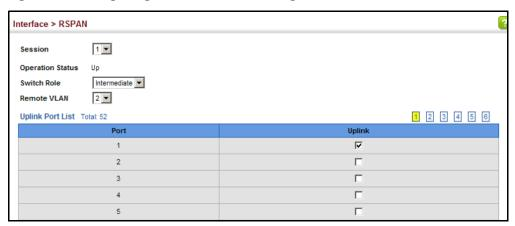
**Figure 38: Configuring Remote Port Mirroring (Destination)**
