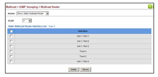
Multicast routers that are attached to ports on the switch use information obtained from IGMP, along with a multicast routing protocol (such as PIM) to support IP multicasting across the Internet. These routers may be dynamically discovered by
