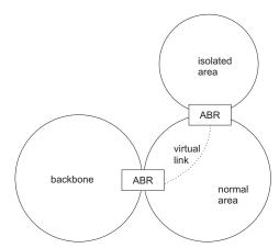
Virtual links can also be used to create a redundant link between any area and the backbone to help prevent partitioning, or to connect two existing backbone areas into a common backbone.
