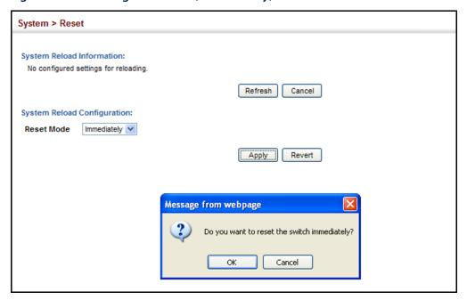
Figure 26: Restarting the Switch (In)
