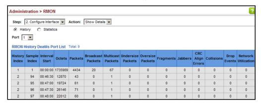
**Configuring RMON** Use the Administration > RMON (Configure Interface - Add - Statistics) page to Statistical Samples collect statistics on a port, which can subsequently be used to monitor the network for common errors and overall traffic rates.
