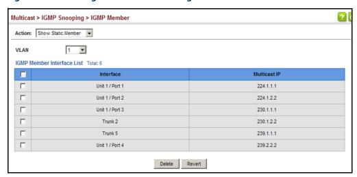
To show the all interfaces attached to a multicast router:
