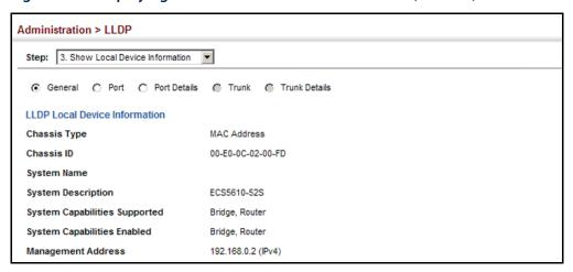
Figure 201: Displaying Local Device Information for LLDP (Port)
