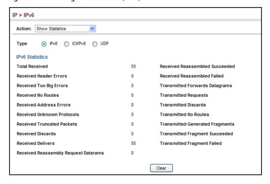
Figure 318: Showing IPv6 Statistics (ICMPv6)
