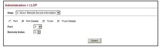
Figure 204: Displaying Remote Device Information for LLDP (Port Details)
