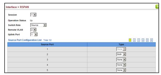
**Figure 37: Configuring Remote Port Mirroring (Intermediate)**
