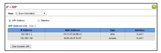
**Displaying ARP** Use the IP > ARP (Show Information) page to display statistics for ARP messages **Statistics** crossing all interfaces on this router.
